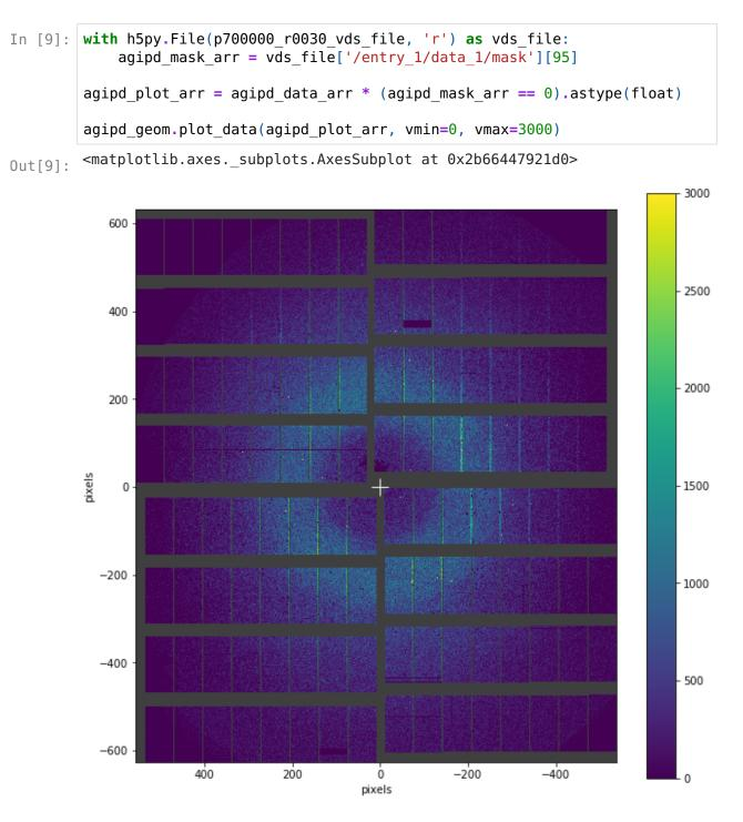
Sometimes a mask from the offline calibration is not enough and an additional, external, mask may be required. For example brighter pixel columns originate from the asics edges which have twice larger pixel size and as a result measure artificially larger intensity. A static mask to exclude these pixels from the analysis can be prepared manually with:
