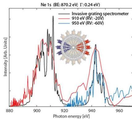
Single shot electron spectra of Neon measured with grating spectrometer (black line), with PES optimized for 910eV and 950eV emitted in one of the two undulator sections
