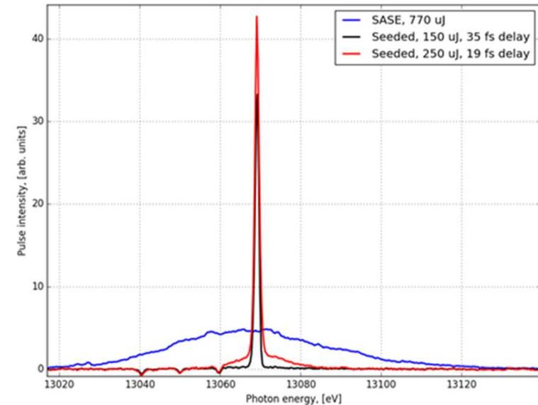
Average self-seeding spectra at 13 keV: nominal SASE operation (blue), setup which was optimized for spectral purity (black), setup which maximizes the spectral flux (red)
