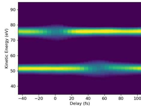
Electron spectra for C1s ionization of  $\text{CH}_3\text{F}$  at 662 and 688 eV, X-ray pulses separated in time by 50fs visualized by perturbation in the electron spectra due to overlap with optical laser pulse.
