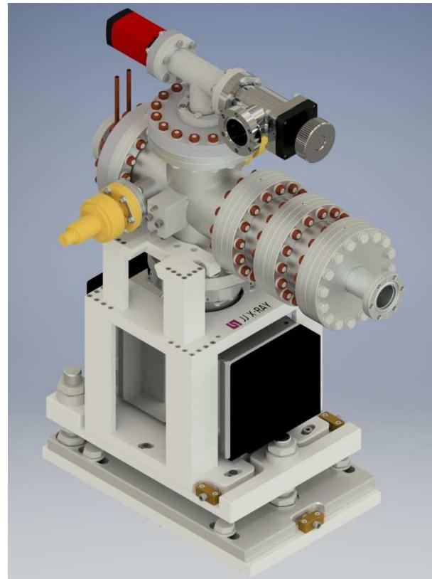
a set of vacuum apertures following a redundant pressure gauge protects the beamline vacuum by means of a fast shutter in case the diamond fails
