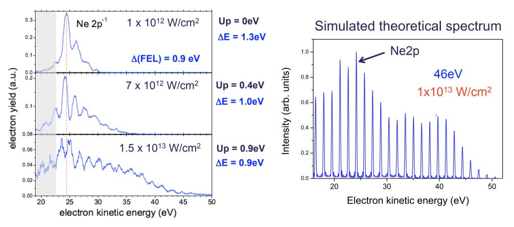
Experiment: bandwidth broadening and jitter (intensity) broadening
