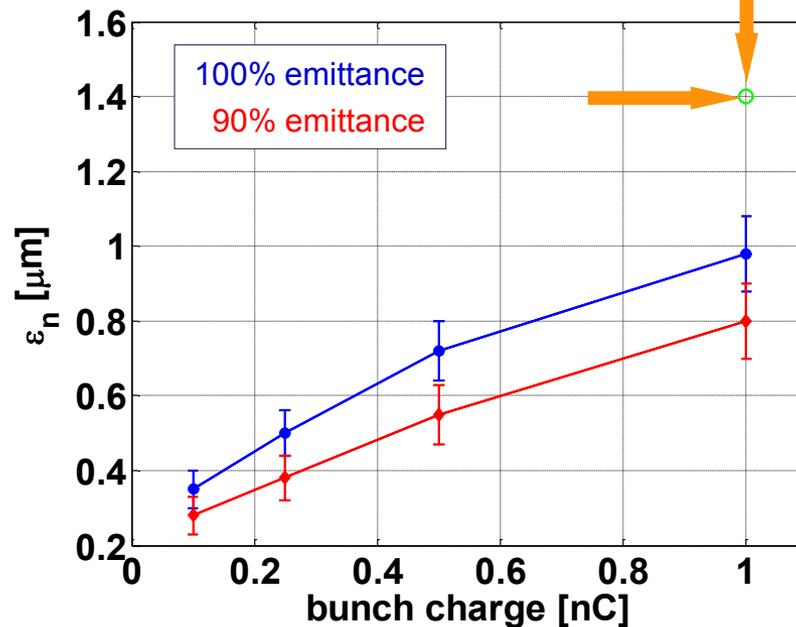
beam emittance vs. BSA size & bunch charge
