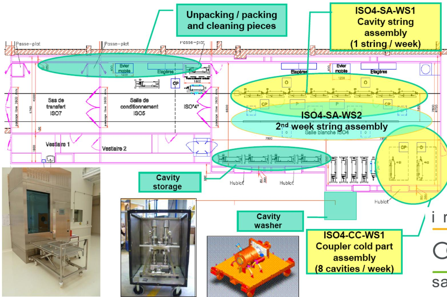
■ All cavities with He tank, the coupler cold parts and the quadrupole-BPM units will be cleaned and dried externally before entering ISO4 area
