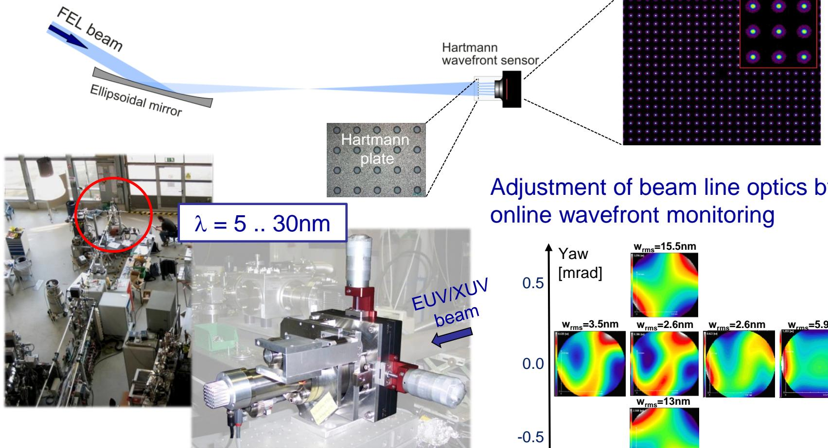
Adjustment of beam line optics by online wavefront monitoring
