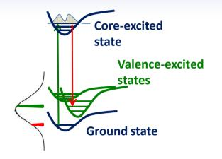
Two-color Raman scattering with seeded source Frequency-domain spectroscopy Pick 2 distinct frequencies within 10 eV SASE bandwidth allows selection of intermediate and final state
