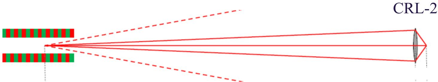
Allows beam sizes 1 – 3  $\mu\text{m}$  with 20-40% efficiency
