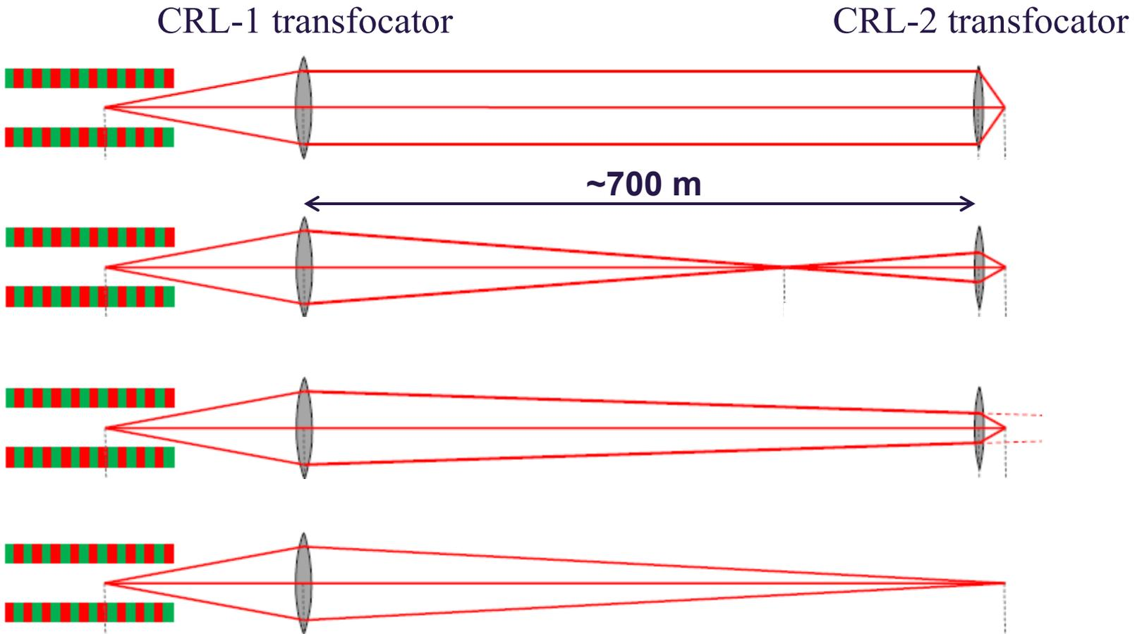
Allows beam sizes on sample from 5 – 200  $\mu\text{m}$  and 80-100% efficiency
