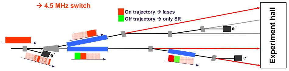
Electron bunch distribution : 27.000 bunches/sec to 3 (5) beamlines; in average 10-20 Hz and ~800 (500) pulses/train; using kicking methods to make bunches lase only in dedicated undulator
