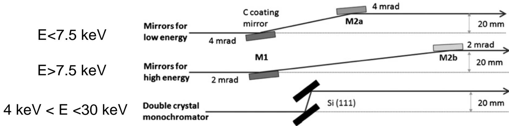
Beamline optics at SACLA. The beam is deflected in vertical direction.
