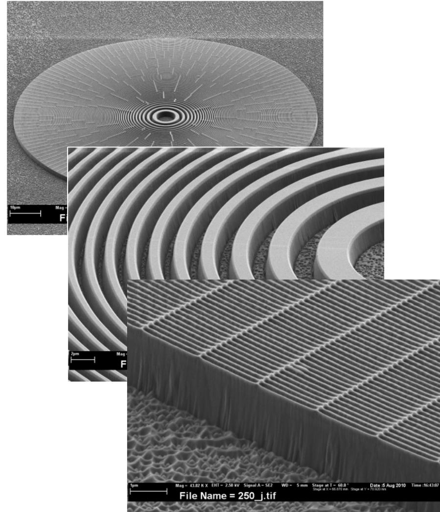
Zone plate structures (100 nm wide, 2  $\mu\text{m}$  high) etched into diamond
