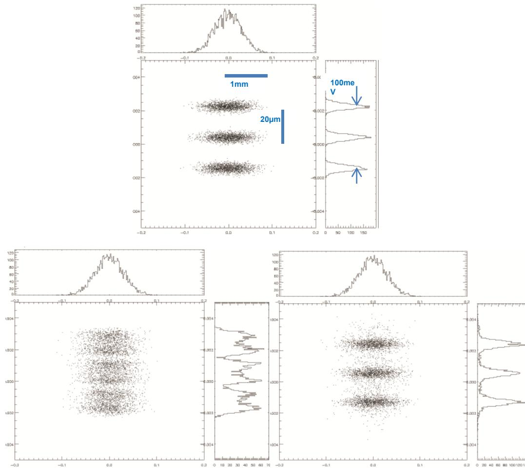
**Figure 8.** Ray trace of operation at 500eV showing the image on the focal plane scintillator i) with no heat, ii) with thermal load corresponding to 100kHz operation and an internally water cooled silicon grating and iii) the same, with the focal plane shifted downstream 58mm to recover the focus as far as possible. Beyond this is the possibility of a cryogenic silicon grating with negligible thermal deformation.
