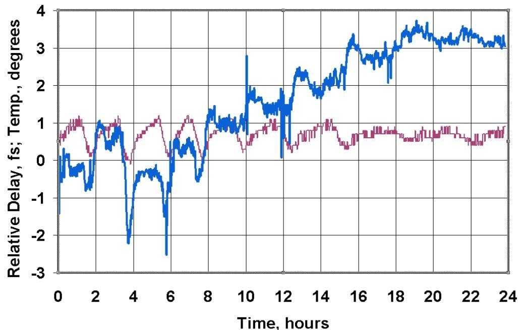
Relative phase delay stability between 2km and 2m
