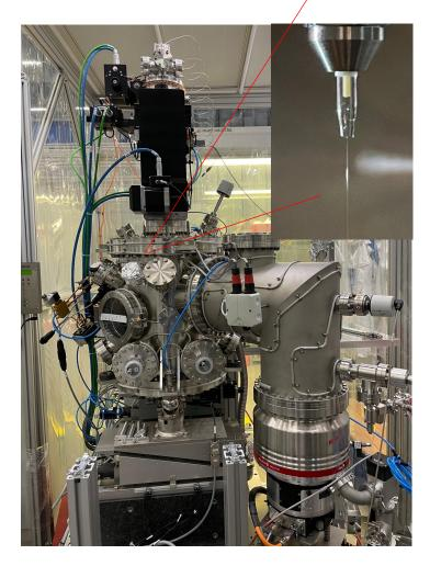
CHEM station is optimized for time-resolved high-resolution RIXS studies of chemical samples in the liquid phase
