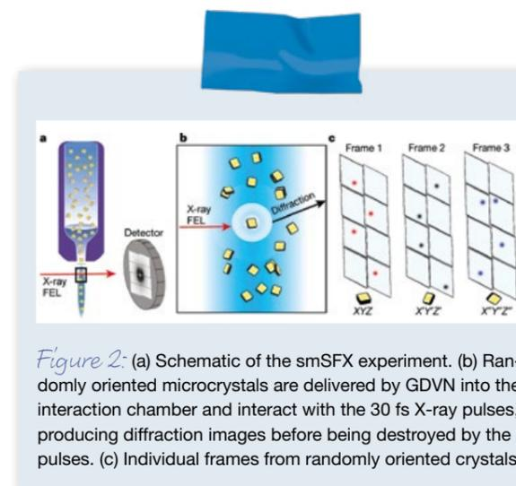
*Figure 2:* (a) Schematic of the smSFX experiment. (b) Randomly oriented microcrystals are delivered by GDVN into the interaction chamber and interact with the 30 fs X-ray pulses, producing diffraction images before being destroyed by the pulses. (c) Individual frames from randomly oriented crystals.
