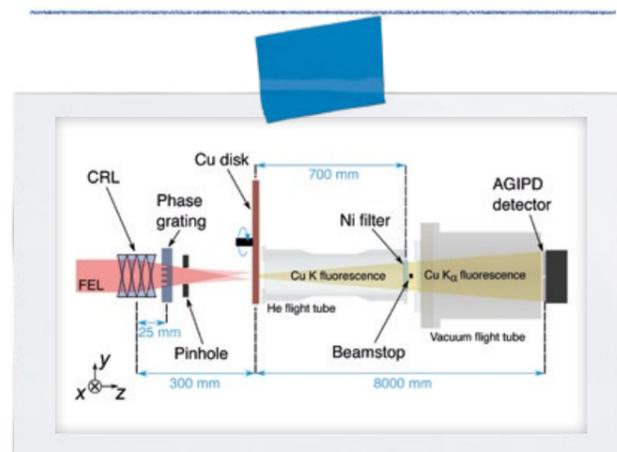
*Figure 1:* Sketch of the experiment setup (CRL: compound refractive lenses, Cu: copper, Ni: nickel, He: helium)
