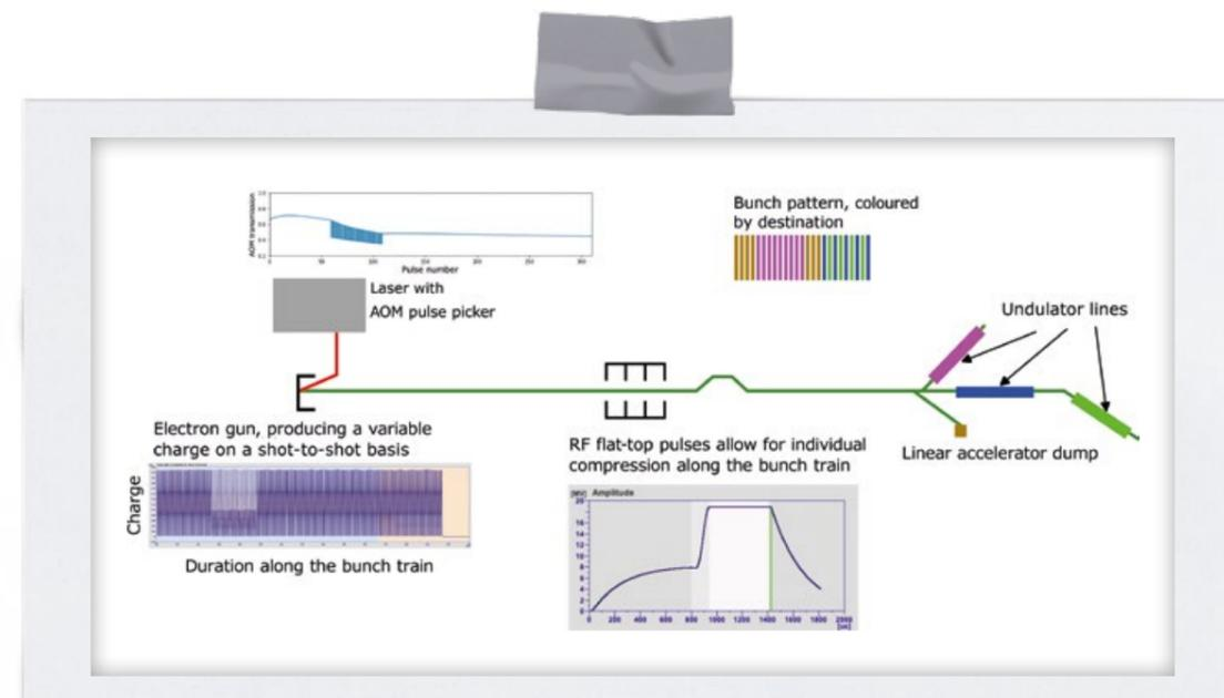
*Figure 1:* Schematic layout of the European XFEL with its electron bunch trains feeding the three FEL undulator lines. The laser AOM absorber located close to the electron gun makes it possible to arbitrarily shape the charge profile of the electron bunches. The modulated RF flat-top pulse allows for individual bunch compression along the train.
