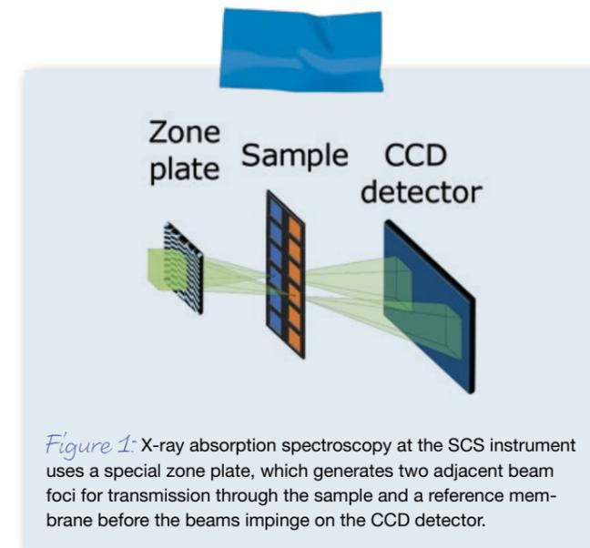
Figure 1: X-ray absorption spectroscopy at the SCS instrument uses a special zone plate, which generates two adjacent beam foci for transmission through the sample and a reference membrane before the beams impinge on the CCD detector.
