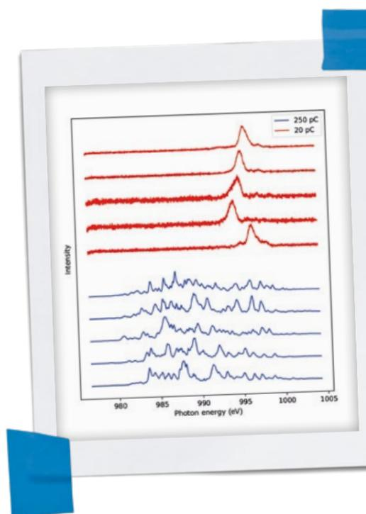
*Figure 2:* Selected X-ray spectra for nominal (250 pC, blue) and low-charge (20 pC, red) electron bunches with optimized electron bunch compression settings
