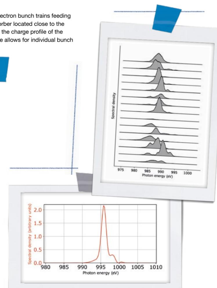
*Figure 3:* Top: Ten consecutive measurements of nearly single-spike X-ray spectra at an averaged pulse energy of 600  $\mu$ J (June 2022). Bottom: Simulation of the spectrum of an ultrashort X-ray pulse produced by over-compression and dispersive settings.
