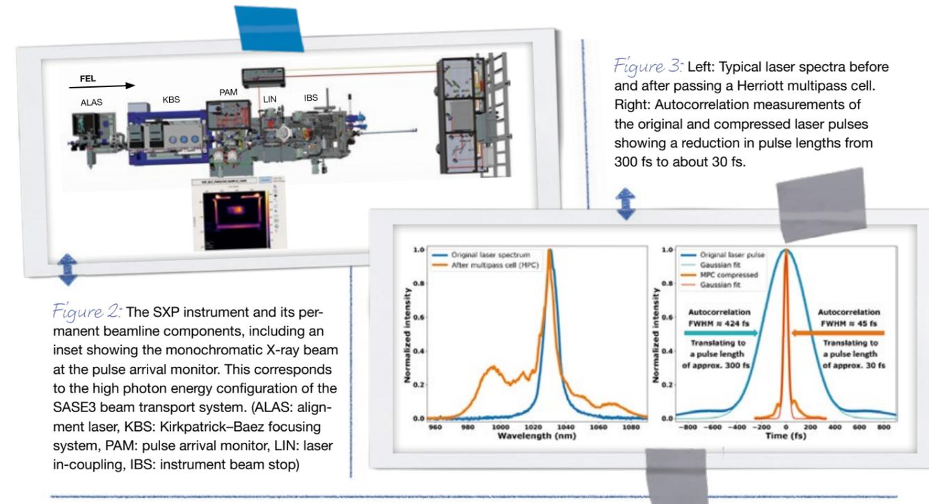
Figure 2: The SXP instrument and its permanent beamline components, including an inset showing the monochromatic X-ray beam at the pulse arrival monitor. This corresponds to the high photon energy configuration of the SASE3 beam transport system. (ALAS: alignment laser, KBS: Kirkpatrick–Baez focusing system, PAM: pulse arrival monitor, LIN: laser in-coupling, IBS: instrument beam stop)
