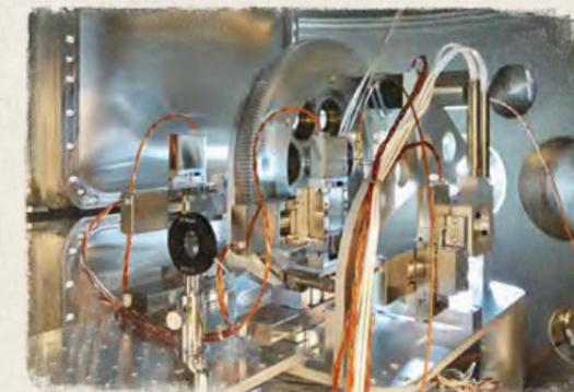
View into the reaction chamber with a revolver for up to six diamond anvil cells in the centre
