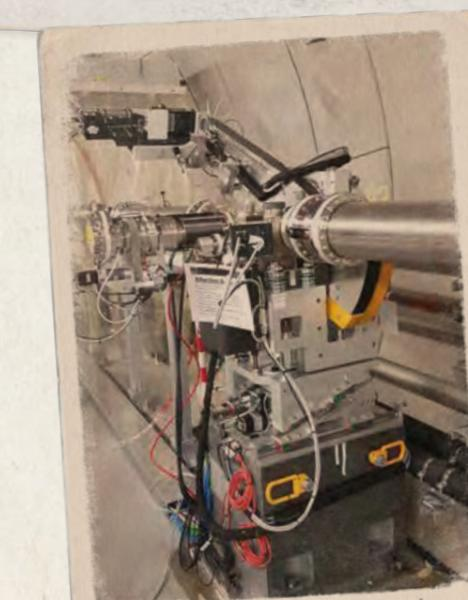
**Figure 3:** HiREX spectrometer with MHz readout capability in the SASE2 beam transport
