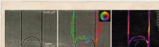
High-speed hard X-ray microscopy movie showing a glass capillary bursting. Left: Image produced from the experiment. Centre: Direction of motion of the debris, showing the spinning glass fragments and details of turbulence in the water. Right: Velocity of the debris in metres per second.
