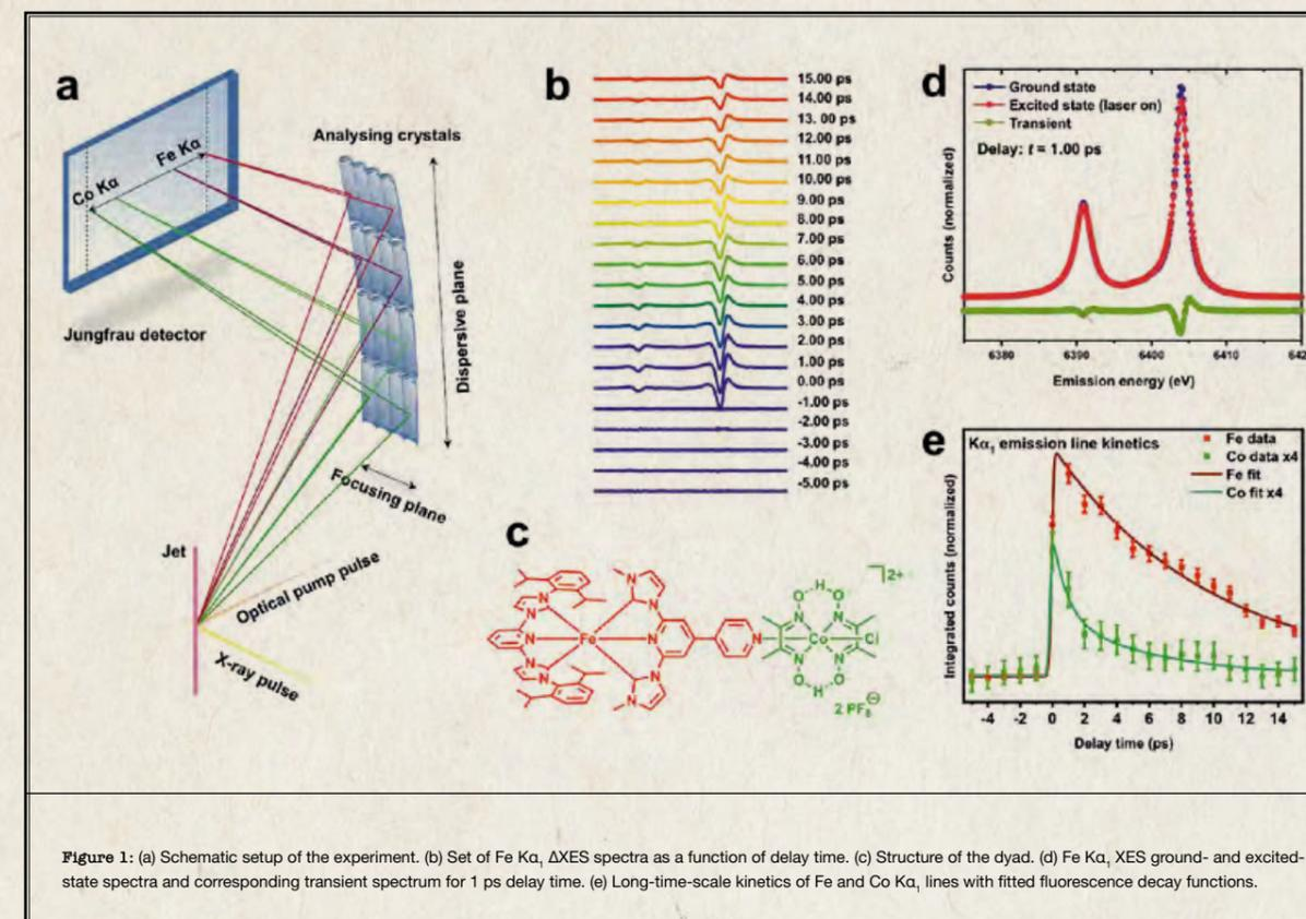
Figure 1: (a) Schematic setup of the experiment. (b) Set of Fe K $\alpha$ ,  $\Delta$ XES spectra as a function of delay time. (c) Structure of the dyad. (d) Fe K $\alpha$ , XES ground- and excited-state spectra and corresponding transient spectrum for 1 ps delay time. (e) Long-time-scale kinetics of Fe and Co K $\alpha$ , lines with fitted fluorescence decay functions.
