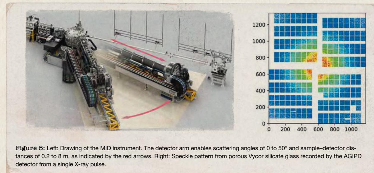
**Figure 5:** Left: Drawing of the MID instrument. The detector arm enables scattering angles of 0 to 50° and sample–detector distances of 0.2 to 8 m, as indicated by the red arrows. Right: Speckle pattern from porous Vycor silicate glass recorded by the AGIPD detector from a single X-ray pulse.
