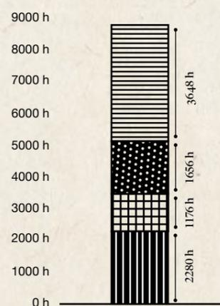
**Figure 1:** Operating hours of the European XFEL accelerator in 2019. The cryogenic system of the accelerator was operated throughout the entire year (8760 h). During this time, 3648 h were dedicated to the delivery of X-ray pulses, 1656 h to facility development, and 1176 h to setup, tuning, and unscheduled access. The remaining 2280 h were scheduled downtime.
