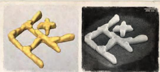
Left: 3D image of a gold sample reconstructed based on the data collected. Right: Reference image of the sample taken with a scanning microscope.
