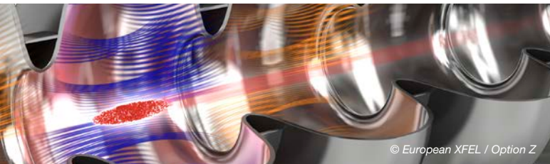
Computer visualisation of the acceleration process in a superconducting cavity resonator
