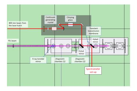
**Figure 7.3:** Tentative schematic layout for the spectral-encoding setup at the SQS end station [adapted from Bionta et al., 2011]. The setup is installed in the two diagnostics chambers downstream the end station (see Figure 7.5). Due to the high divergence of the FEL beam, the possibility of refocusing is foreseen. The relative position of the refocusing mirror, the two holed OL mirrors and the transienttransmission membrane can be adjusted to optimal operation conditions.
