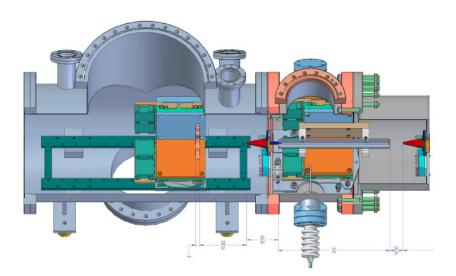
*Figure 5.2:* Design of the controlled-molecules setup for CAMP at LCLS provided by Küpper et al. (CFEL Hamburg). The large flanges are DN 250 CF in this particular setup and the measures given in the figure are in millimetres.
