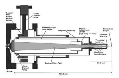
Figure 3.3.6: Scheme of the HReTOF spectrometer [see Hemmers et al., 2010]
