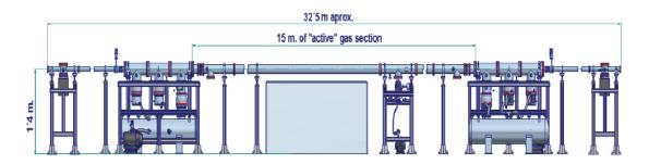
*Figure 2.5:* Schematic view of the gas cell attenuator on the SASE3 beamline [TDR-BT\_2012]
