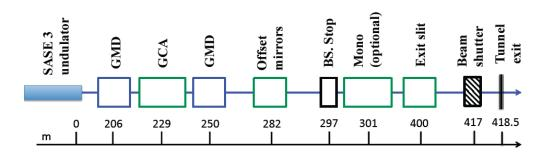
Figure 2.4: Schematic presentation of the main components for the SASE3 beamline
