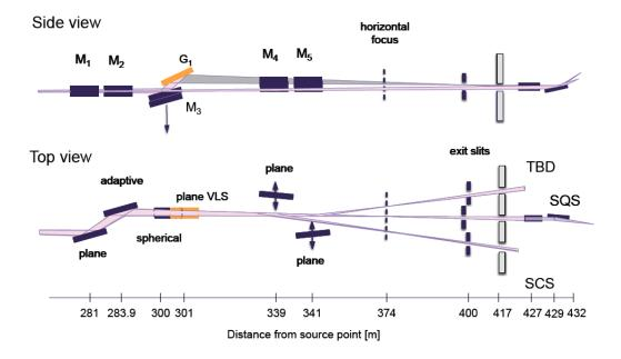
*Figure 2.6:* Schematic layout of the SASE3 beamline including the VLS monochromator [from TDR-BT\_2012]
