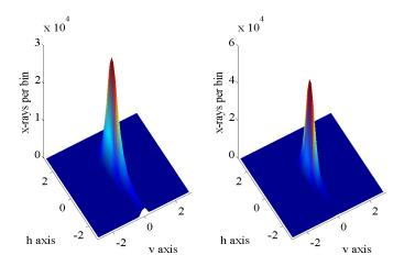
**Figure 3.2.13:** 2D image of the AQS focal spot at 1 keV (left) and 2.5 keV (right) incident photon energy. The beam is optimally focused along the vertical plane, whereas the focusing in the horizontal plane shows slight divergence-dependent aberration.
