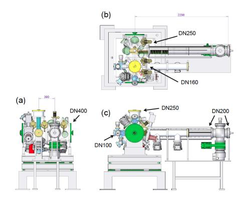
*Figure 3.3.2:* AQS experiment chamber: (a) side view, (b) top view and (c) front view. Some of the principal distances and port size parameters are indicated. For convenience the tilt of the experiment chamber imposed by the KB optics is not represented.
