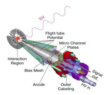
*Figure 3.3.14:* Design sketch of the high-efficiency eTOF spectrometer [Viefhaus et al., in preparation]
