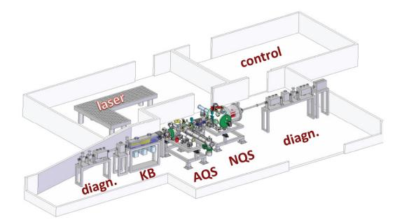
*Figure 3.1.2:* Layout of the SQS experiment area with the control room and SQS laser hutch
