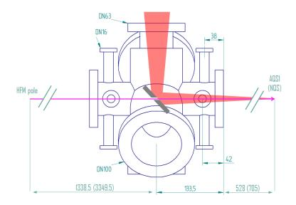
*Figure 6.2:* Sketch of the laser in-coupling chamber (LIC) including distances between last KB mirror pole, in-coupling mirror, and interaction point for the AQS (NQS) chamber. Besides the OL coupling, the vessel hosts two sets of four motorized blades for beam baffling.
