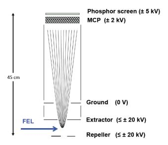
Figure 3.3.7: Schematic view of the VMI spectrometer
