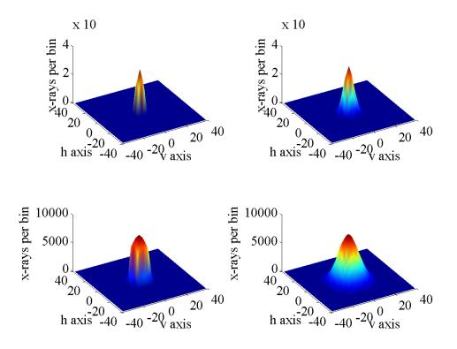
**Figure 3.2.10:** 2D representation of the intensity profile in the AQS interaction point (F1) for different photon energies and detuning angles. Top left: hv = 0.5 keV, detuning set to 10 µm spot size. Top right: hv = 2.5 keV, detuning set to 10 µm spot size. Bottom left: hv = 0.5 keV, detuning set to 20 µm spot size. Bottom right: hv = 2.0 keV, detuning set to 20 µm spot size. At low photon energies, the effect of the finite size of the mirror is quite evident in the spot shape.
