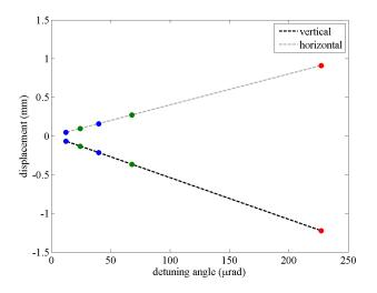
*Figure 3.2.12:* Horizontal and vertical displacements of the focal spot in the transverse plane are shown as a function of incidence angle detuning.
