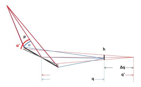
**Figure 3.2.8:** Schematic representation of the spot size detuning by detuning of the incidence angle. The image distance changes with the incidence angle according to Equation (3.3). If the change in the image distance is small, the beam section in the original image position h is just the projection of the footprint on the mirror f, and its size is proportional to the image displacement dq/q (Equation 3.4).
