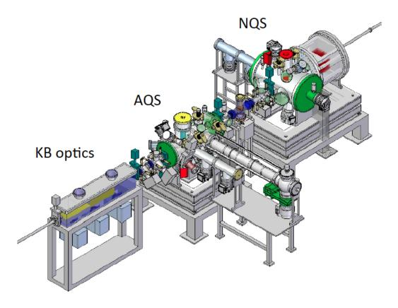
*Figure 3.1.4:* Global view of the SQS experiment station with the AQS and NQS vacuum chambers and the KB focusing optics
