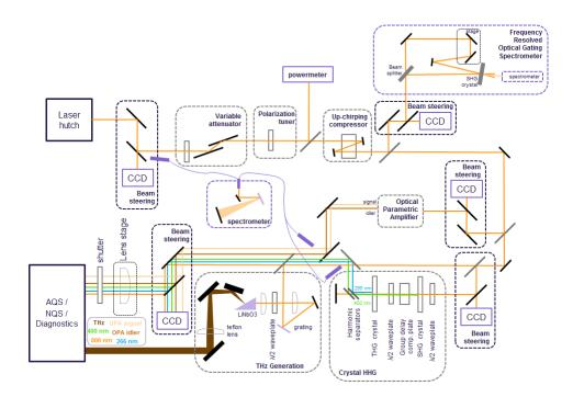
**Figure 6.1:** Tentative optical layout of the SQS laser operation system. Different colours are used to identify different categories of devices: control devices for beam properties (grey boxes), beam steering (black boxes), and monitor devices for beam properties and diagnostics tools (purple boxes).
