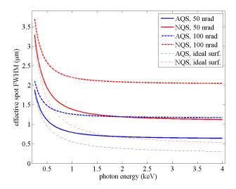
**Figure 3.2.6:** Expected spot size in the main interaction region of AQS (F1) and NQS (F2) assuming a 50 nrad and a 100 nrad RMS slope error. Effective spot FWHM is calculated as sqrt (FWHM<sub>vert</sub> x FWHM<sub>horiz</sub>). The spot size calculation includes geometric optics, diffraction effects, and slope error effects. As a reference, the spot size produced by an ideal surface (neglecting slope error effects) is represented.
