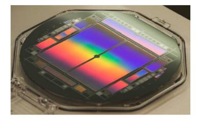
**Figure 3.3.19:** Photograph of a pnCCD sensor wafer without readout electronics and mechanical components. The two sensitive sensor areas with a size of 512 x 1024 pixels are clearly visible as large rectangular areas. The hole in the centre of the device provides sufficient space for the not-scattered central beam to pass through the sensor [Strüder et al. 2010].
