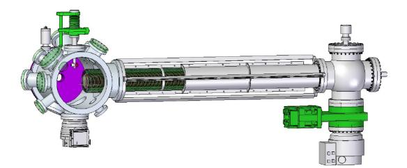
Figure 3.3.11: 3D CAD drawing of a magnetic bottle
