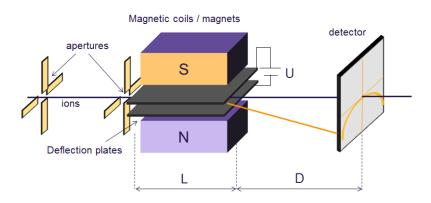
*Figure 3.3.15:* Operation principle of the Thompson spectrometer. An imaging detector collects the ions. The two dimensions of the detector map the charge-to-mass ratio and the velocity (energy) of the ions simultaneously.
