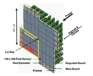
*Figure 3.3.17:* Conceptual drawing of the DSSC detector illustrating the sensor geometry and arrangement of the front-end electronics [Porro et al., 2010]
