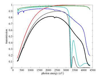
**Figure 3.2.3:** Total transmission of the SASE3 beamline and the contributions of the individual components as a function of photon energy. Blue: Reflectivity of  $B_4C/Cr$  bilayer on a Si substrate.  $B_4C$  thickness is 12 nm, Cr thickness is 120 nm. Surface roughness is set to 1 nm for both layers and the substrate. Green: Reflectivity of  $B_4C$  single layer (50 nm thickness, 1 nm roughness). The reflectivity values are
