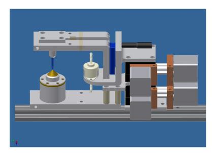
Figure 5.1: Scheme of the compact liquid-jet setup (Microliquids GmbH)
