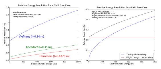
**Figure 3.3.5:** (a) Relative energy resolution for different TOF spectrometers. (b) Decomposition of the energy resolution into the contribution from the flight length  $\Delta l$  and the timing uncertainties  $\Delta t$ .
