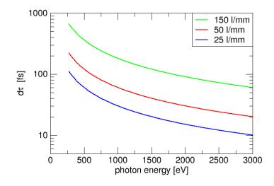
*Figure 2.8:* Pulse stretching for a 4-sigma illuminated grating of 500 mm length [TDR-BT\_2012]
