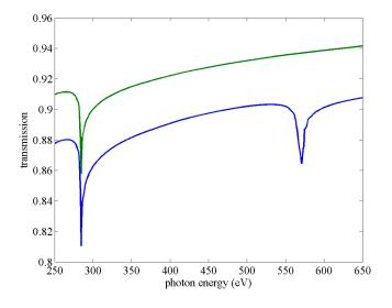
**Figure 3.2.4:** B<sub>4</sub>C/Cr bilayer (blue) and B<sub>4</sub>C single-layer (green) reflectivity in the C-1s and Cr-2p edge regions, calculated as in Figure 3.2.3
