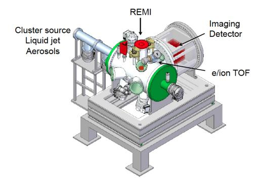
Figure 3.3.12: Schematic view of the NQS experiment chamber
