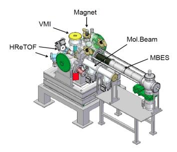
Figure 3.3.1: Schematic view of the AQS experiment chamber
