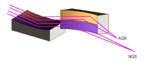
**Figure 3.2.1:** Schematic representation of the KB mirror system design. For both vertical and horizontal focusing, two stripes with fixed-profile ellipses are shaped onto the same substrate, one beside the other, directly focusing the SASE3 undulator source in the two main interaction points F1 (AQS) and F2 (NQS).
