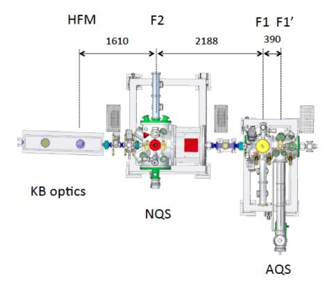
*Figure 3.1.6:* Top view of the SQS experiment station with the NQS and AQS vacuum chambers and the KB focusing optics. The order of the AQS and NQS chamber is inverted with respect to the configuration shown in Figure 3.1.5.
