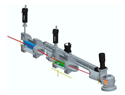
*Figure 3.3.10:* Sketch of the 1D imaging XUV spectrometer. Distance from source to imaging cylindrical mirror (blue): 940 mm; radius of cylindrical grating (green): 20 m; movement of grating: 450 mm x 10 mm; groove frequency of grating: 600 /mm.
