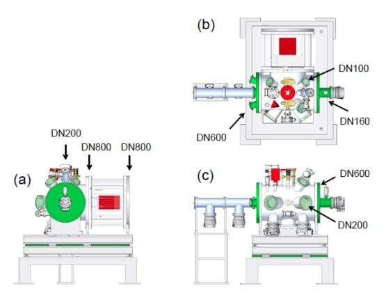
*Figure 3.3.13:* NQS experiment chamber: (a) side view, (b) top view, and (c) front view. Some of the principal distances and port size parameters are indicated.
