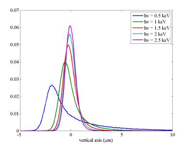
**Figure 3.2.14:** Vertical profiles of the monochromatic beam in the AQS focus for different photon energies. The profiles are normalized to the transmission of the optics.
