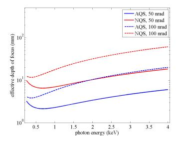
**Figure 3.2.7:** Expected depth of focus in the main interaction region of AQS (F1) and NQS (F2) assuming a 50 nrad and a 100 nrad RMS slope error. The depth of focus along the beam axis is defined here as twice the distance between the focal point and the point where the intensity is half of the value in the focus.
