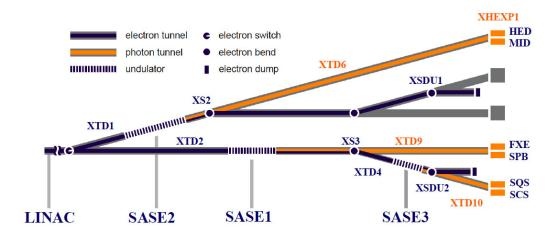
Figure 2.1: Electron and photon beam distribution for the European XFEL
