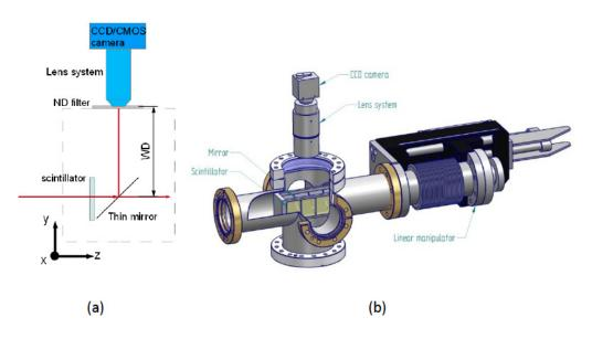
*Figure 7.6:* (a) Optical imaging system and (b) mechanical model for the imaging station [from CDR (WP74): Imaging Stations for Invasive Diagnostics].
