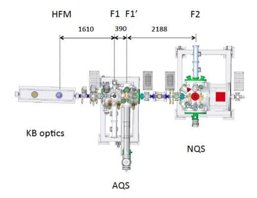
*Figure 3.1.5:* Top view of the SQS experiment station with the AQS and NQS vacuum chambers and the KB focusing optics
