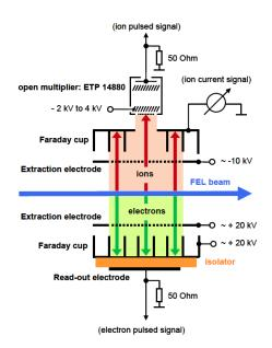
Figure 7.1: Schematic diagram for the XGMD used at the SQS scientific instrument
