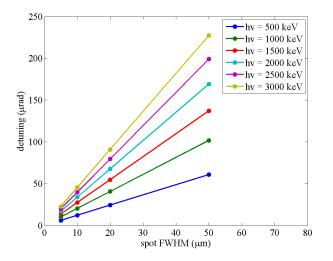
**Figure 3.2.9:**  $\alpha' - \alpha$  dependence on the spot size h in the F1 interaction point for different photon energies. The detuning values are calculated for the vertical mirror VFM. According to Equations (3.2) and (3.3), the detuning of HFM has to be ~ 0.4% lower.
