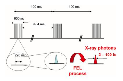
Figure 2.3: Pulse structure for the operation mode of the European XFEL
