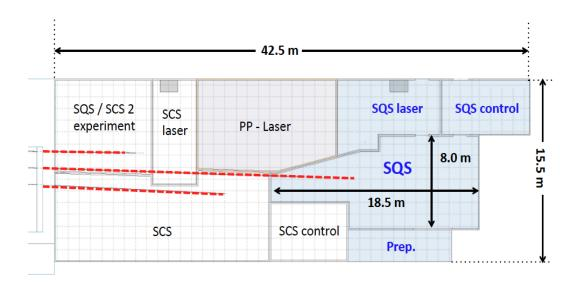
*Figure 3.1.1:* Layout of the SQS experiment area, the control room, and the preparation area on the floor space behind the SASE3 undulator
