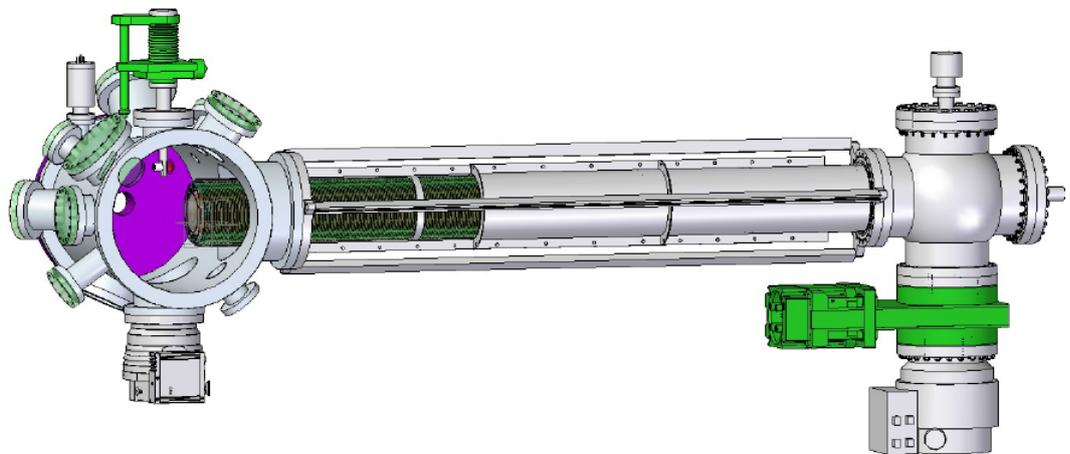
*Figure 3.3.11: 3D CAD drawing of a magnetic bottle*
