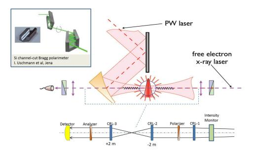
**Figure 3-12.** Schematic of vacuum birefringence experiment. The PW-class OL beam propagates through focus from left to right, counter to the European XFEL beam (right to left). Silicon channel-cut Bragg crystal polarimeters (inset) are used in crossed polarizer–analyser geometry. Beryllium compound refractive lenses (CRL) are used to ensure large (200  $\mu$ m) parallel beams at the Si polarimeters, with a tight focus (< 200 nm diameter) to overlap the OL laser focus (~ 2  $\mu$ m).
