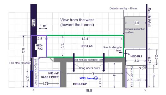
*Figure 8-2.* Rear view of the HED-EXP area looking from the west wall and indicating the infrastructure room adjacent to the experiment room
