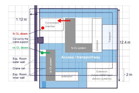
Figure 8-8. Layout of HED-LAS room at 4.8 m height
