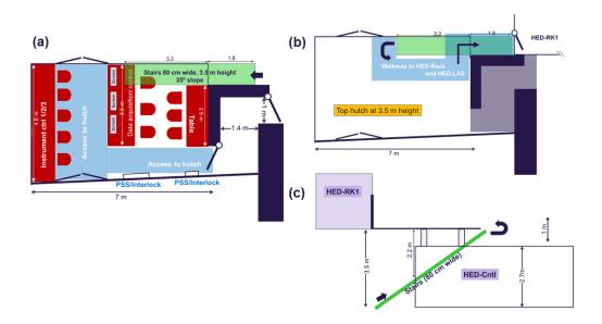
*Figure 8-7.* Layout of the HED-CTR room: (a) Top view. (b) Top view of the ceiling level of HED-CTR, which will be used as a footpath to access the HED rack rooms and HED-LAS in the top hutch. (c) Side view showing how the stairs will be arranged.
