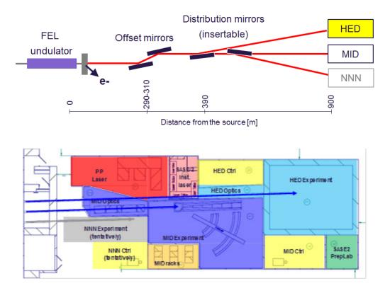
**Figure 2-1**. Sketch of the SASE2 beam transport system (top) and of the floor layout of SASE2 instruments HED (blue), MID (purple), and NNN (grey) inside the experiment hall (bottom). Red areas indicate laser rooms while green areas mark laboratory space.
