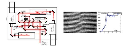
*Figure 6-4.* (Left) Schematic setup of the VISAR system installed at Laboratoire pour l'Utilisation des Lasers Intenses (LULI) in Palaiseau, France. (Right) Fringe pattern and velocity profile obtained with VISAR in isentropic experiments, courtesy E. Brambrink.
