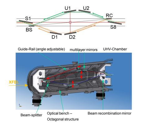
**Figure 5-11.** (Top) Schematic drawing of the optical layout of the SDU. The X-ray beam is divided geometrically at the beam splitter (BS). The mirrors U1, U2, D1, and D2 can be moved along the beam direction to change the delay *τ*. The lower (orange) beam will be reflected by the recombination mirror (RC) onto the last mirror S8. (Bottom) Mechanical layout of the optical bench with the optomechanical components.
