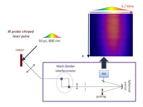
Figure 6-2. Schematic layout of FDI diagnostic system
