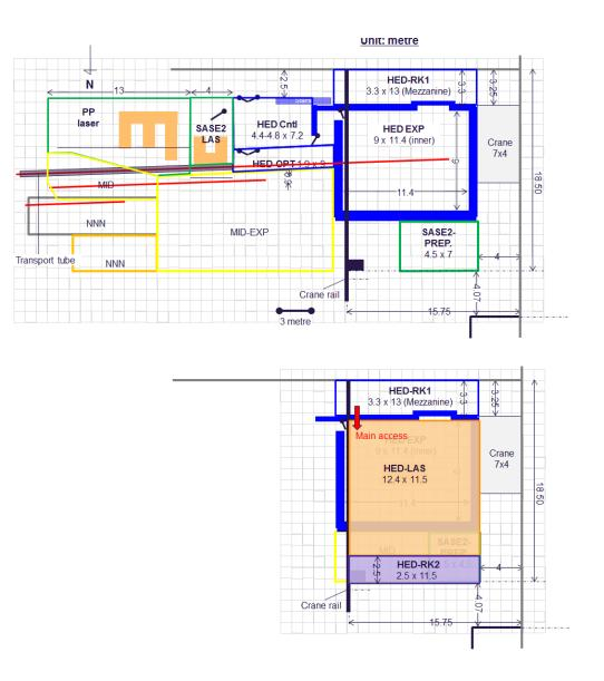
**Figure 8-1.** Layout of the SASE2 area inside the experiment hall XHEXP. Shown are only the HED-relevant rooms. One square indicates  $1 \times 1 m^2$ . (Top) Experiment floor. HED-RK1 is at the mezzanine level at 3.5 m height. (Bottom) HED-LAS and HED-RK2 at 4.8 m height above the floor.
