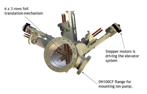
*Figure 5-13.* Mechanical design and concept of the three-arm attenuator. Design provided by JJ X-Ray, Denmark.
