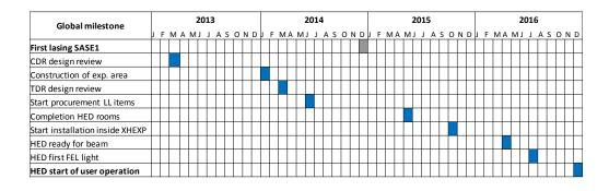
*Figure 9-1.* Outline of schedule for the construction of the European XFEL HED instrument
