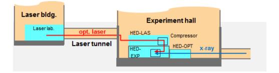
**Figure 6-5.** Schematic presentation of the laser building adjacent to the experiment hall XHEXP and of the laser beam transport from the laser tunnel, first into the HED-LAS room and then after compression to the experiment area.
