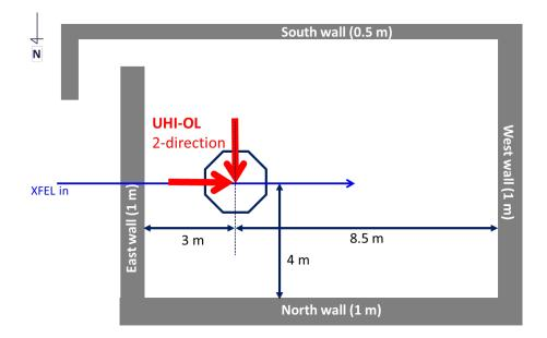
*Figure 8-5.* Geometry of HED-EXP for the radiation simulations. The two red arrows indicate the two alternative perpendicular and collinear geometries.
