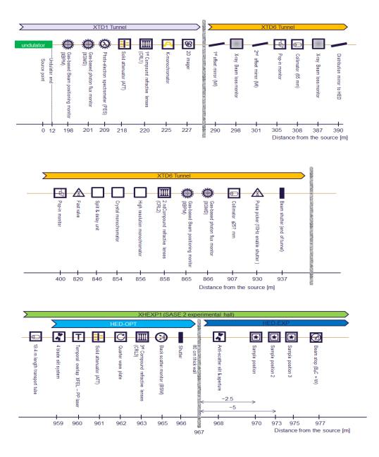
Figure 5-4. Details of HED X-ray devices, including source distances
