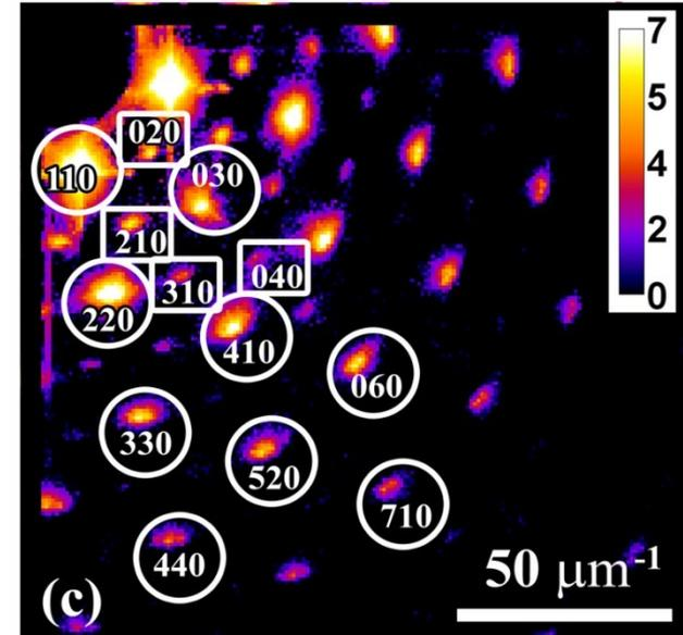
X-ray diffraction pattern of the **experiment A** measured at room temperature.
