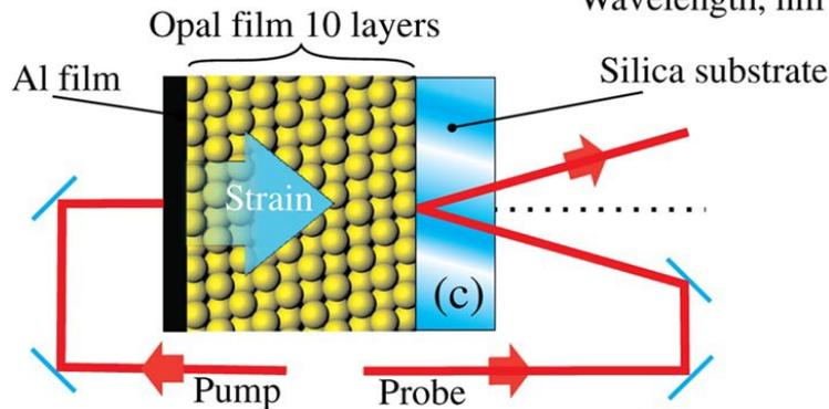
Set up for pump-probe experiment
