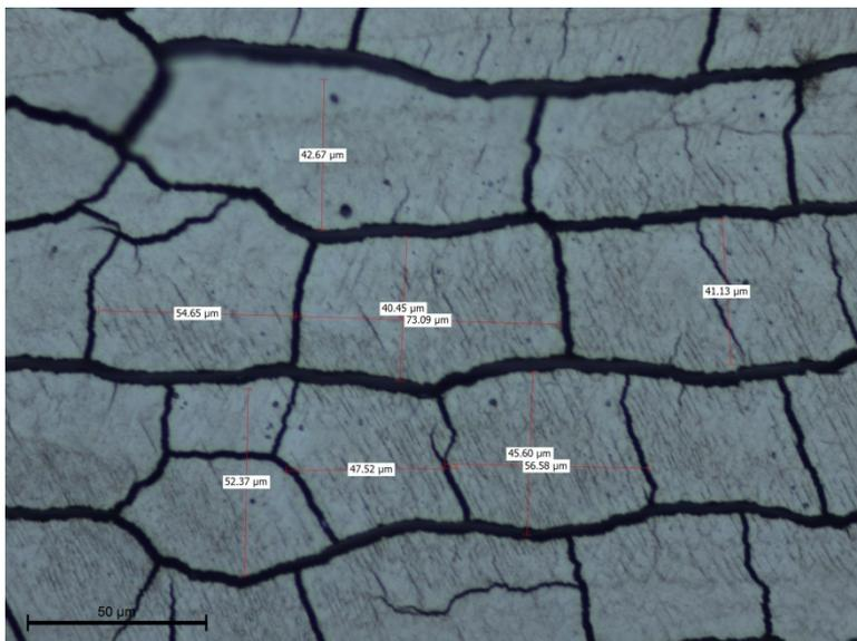
Distance between cracks around 50 μm
