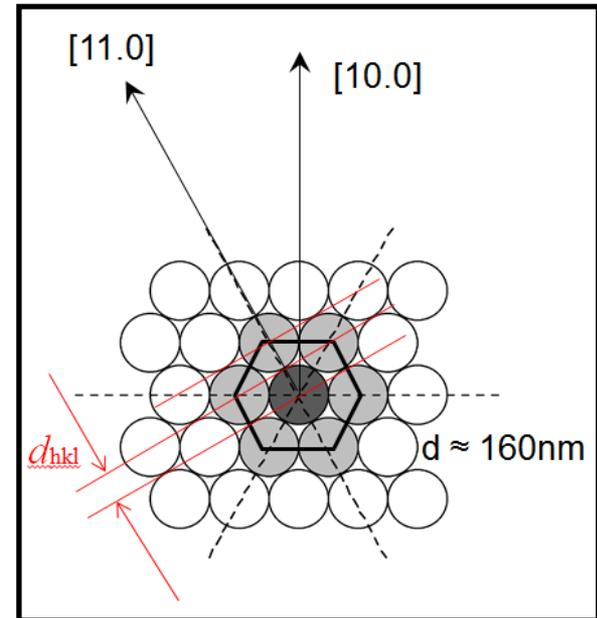
Crystallographic directions in colloidal crystal
