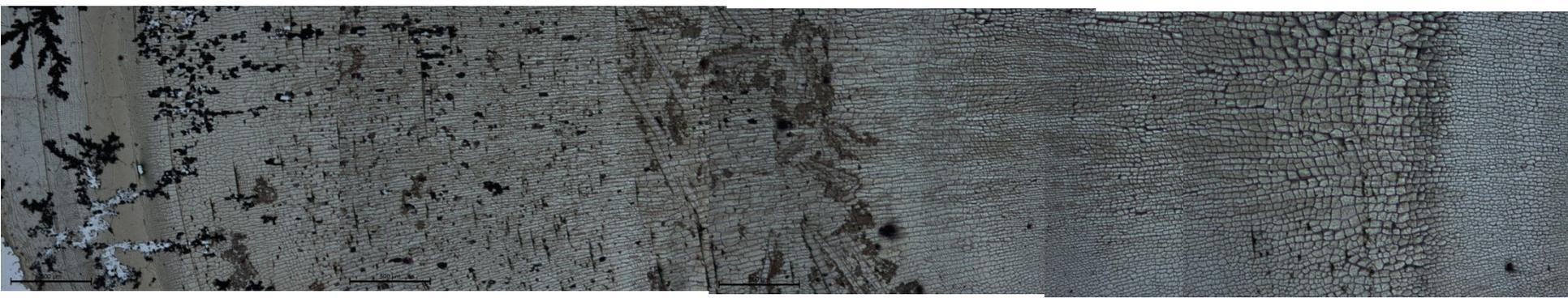
Top to middle of sample. At the top the sample is quite damaged, but the middle region with a lot of layers and larger area's between the cracks has higher quality.
