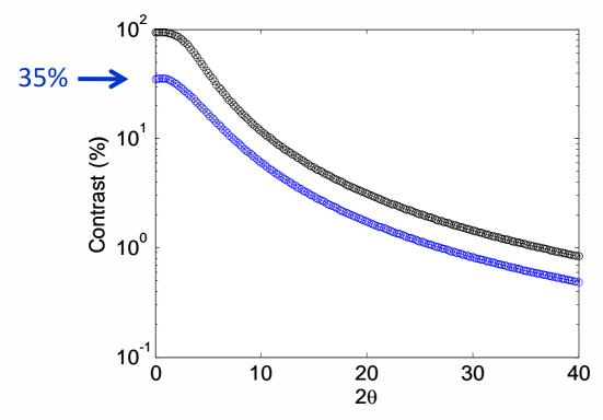
Troika: 10mu beam, 8keV Si(111), 22micron pixels 2.3m sample-CCD dist. 0.1mm sample thickness
