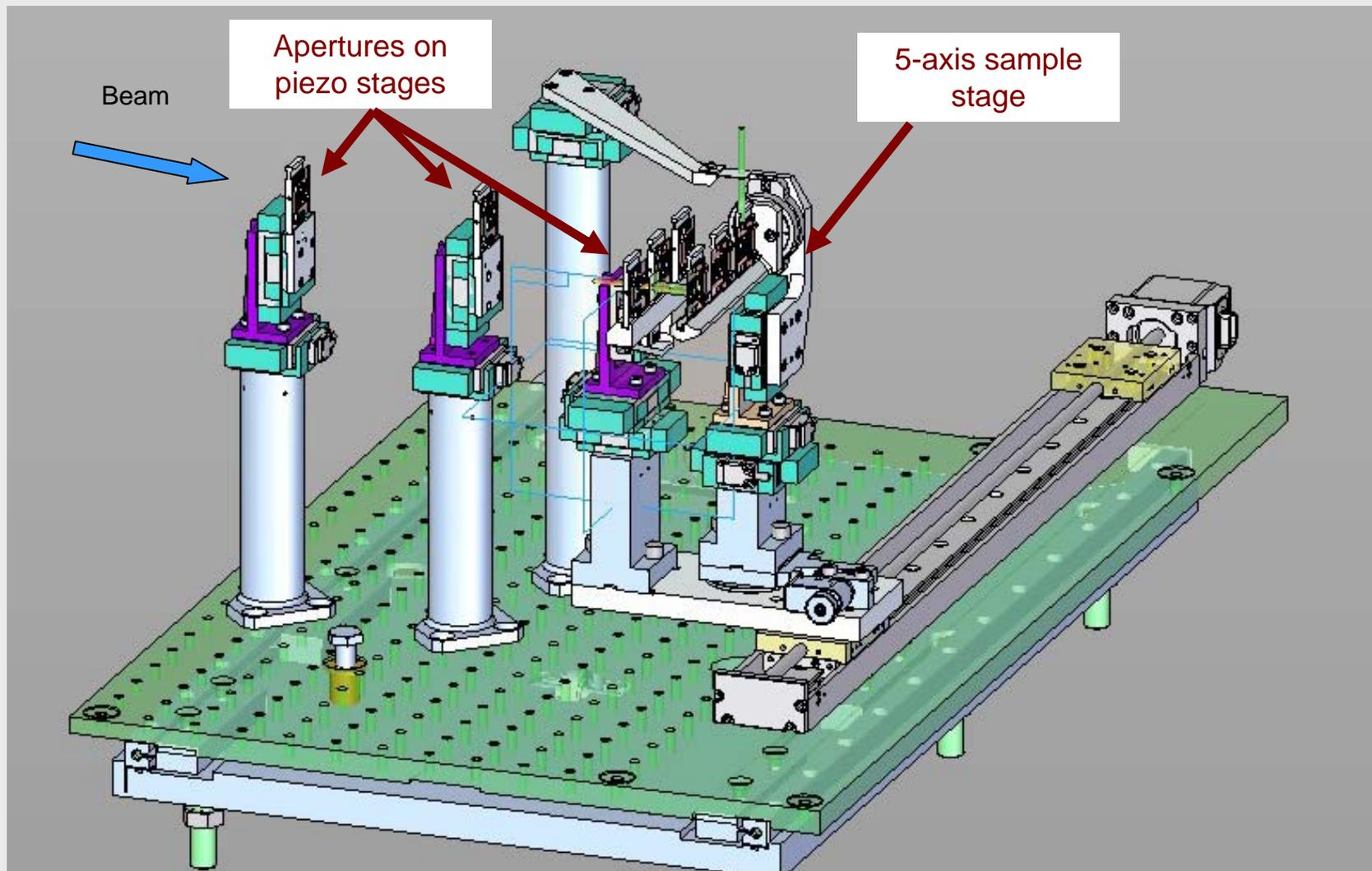
Many apertures are needed to measure signal at small angles
