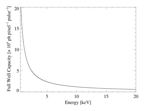
**Figure 23.** Anticipated full well capacity of the AGIPD sensor as a function of incident photon energy as estimated from the 1  $\times$  10<sup>4</sup> photons/per pixel/pulse at 12 keV specification. (Figure courtesy of Markus Kuster, European XFEL.)
