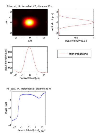
**Figure 12.** Intensity and phase of the 12 keV beam in the focal plane from a Palladium-coated KB pair (modelled as a lens with aberrations that correspond to realistic height errors) with ~ 35 m focal distance and an aperture governed by the 800 mm length mirrors The total transmission of the system is about 76%.
