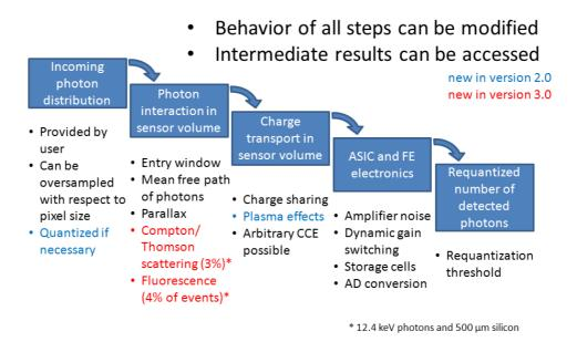
**Figure 6.** HORUS detector simulation processing chain. Image courtesy of Julian Becker, DESY, Hamburg.
