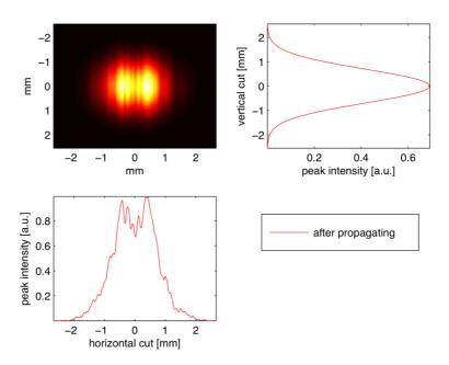
**Figure 10.** Modelled 12 keV European XFEL beam in the optics hutch prior to the 1 μm KB mirrors after propagating from the source via the horizontal offset mirrors (HOMs), including realistic estimates of height error for the HOMs.
