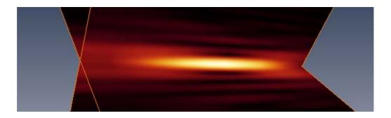
**Figure 18.** Longitudinal profile of the nominally 100 nm focal spot for 12 keV radiation and Pd-coated mirrors. The longitudinal dimension is 1 mm. Note again the long depth of focus.
