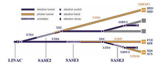
**Figure 3.** Layout of the European XFEL accelerator, undulator, and X-ray beam transport systems. Note that the SPB instrument is located after the SASE1 undulator. Figure sourced from [23].
