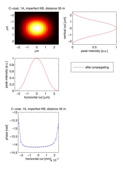
Figure 11. Intensity and phase of the 12 keV beam in the focal plane from a carbon-coated KB pair (modelled as a lens with aberrations that correspond to realistic height errors) with ~ 35 m focal length and an aperture governed by the 800 mm length mirrors. The total transmission of the system is about 41%.
