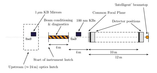
**Figure 7.** Conceptual design of the optical layout of the SPB instrument. Note well the upstream optics hutch, which is to be located as far upstream as possible on the experiment hall floor. This long distance is necessary to deliver the ~ 1 μm spot requested by the single particle imaging community. Figure 8 details this approximately to scale.
