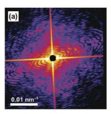
Figure 2. An example of a coherent diffraction pattern from a single-celled organism with strong signal spanning orders of magnitude of dynamic range. Figure originally published in A.P. Mancuso et al., New J. Phys., 12, 035003 (2010).
