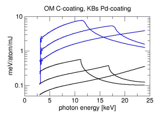
**Figure 9.** Deposited energy per atom for the offset and the KB mirrors for increasingly steep graze angles. The black lines are for the offset mirrors (Carbon coated), the blue lines for the Pd-coated KB mirrors. Figure taken from [23].
