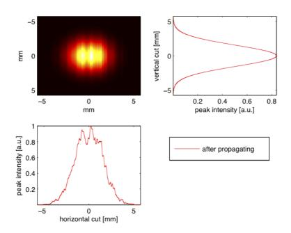
Figure 14. Modelled 5 keV European XFEL beam in the optics hutch prior to the 1 µm KB mirrors after propagating from the source via the horizontal offset mirrors (HOMs), including realistic estimates of height error for the HOMs.
