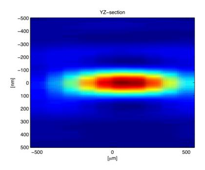
**Figure 20.** Sections of the 5 keV, 100 nm beam focus shown perpendicular to the direction of propagation. Note again the large depth of focus, here a few hundreds of microns.
