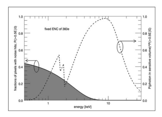
**Figure 22.** Efficiency of the AGIPD detector and fractions of pixels with false hits as a function of photon energy. This plot is an approximation based on preliminary data. (Figure courtesy of Julian Becker and Heinz Graafsma, DESY.)
