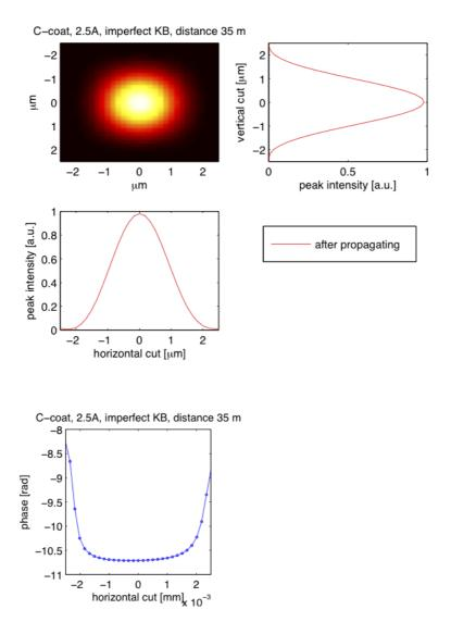
**Figure 15.** Intensity and phase of the 5 keV beam in the focal plane from a carbon-coated KB pair (modelled as a lens with aberrations that correspond to realistic height errors) with ~ 35 m focal distance and an aperture governed by the 800 mm length mirrors. The total transmission of the system is about 55%.
