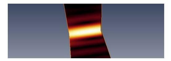
Figure 13. Longitudinal profile of the nominally 1 µm focal spot for 12 keV radiation and Pd-coated mirrors. The longitudinal dimension of the intensity profile shown is 14.5 mm. Note the extremely long depth of focus (even longer than shown here), which is of great benefit for the coherent imaging of injected samples.
