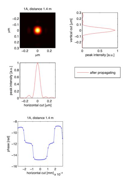
**Figure 17.** Intensity and phase of the 12 keV beam in the focal plane from a Palladium-coated KB pair (modelled as a lens with aberrations that correspond to realistic height errors) with 1.4 m focal distance and an aperture governed by the 550 mm usable length mirrors. The total transmission of the system is about 48%.
