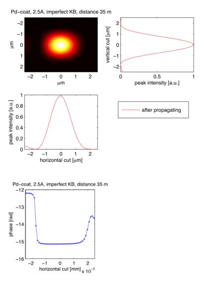
Figure 16. Intensity and phase of the 5 keV beam in the focal plane from a Pd-coated KB pair (modelled as a lens with aberrations that correspond to height errors) with ~ 35 m focal distance and an aperture governed by the 800 mm length mirrors. The total transmission of the system is about 74%.
