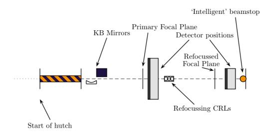
**Figure 21.** Refocusing option. The length of the entire instrument can benefit from being slightly longer in the refocusing case, in order to fit the additional optics and interaction region in the instrument hutch.
