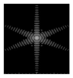
**Figure 1.** A simulated diffraction pattern around a Bragg peak produced by an icosahedral-shaped crystal. The signal shown here (on a log scale) spans more than three orders of magnitude. Weaker signal from the simulation has been suppressed by a modelled noise-floor.
