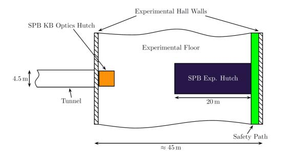
Figure 8. Approximate scale sketch of the location of the SPB optics hutch with respect to the SPB experiment hutch and the experiment floor. The beam propagates from left to right. The KB optics hutch is located approximately 24 m upstream of the interaction region, i.e., as far upstream as possible while still on the experiment floor. The experiment floor continues in both directions perpendicular to the beam propagation.
