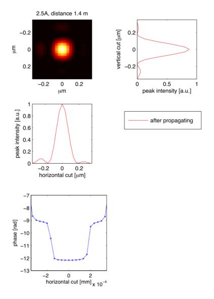
Figure 19. Intensity and phase of the 5 keV beam in the focal plane from a Palladium-coated KB pair (modelled as a lens with aberrations that correspond to realistic height errors) with 1.4 m focal distance and an aperture governed by the 550 mm usable length mirrors. The total transmission of the system is about 22%.
