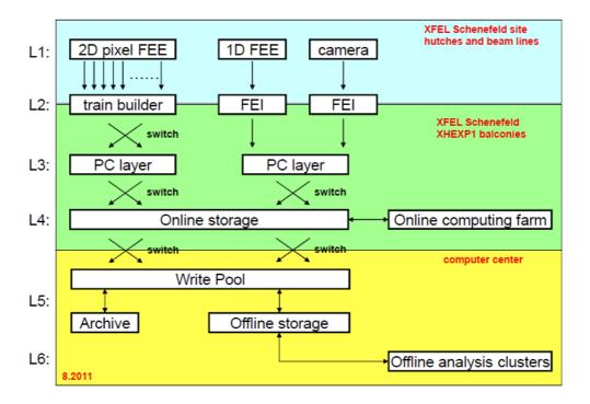
Figure 24. Common XFEL data handling architecture
