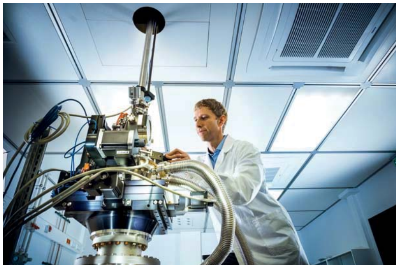
Figure 2 Group member James Moore installs the sample handling device for the MID compact pulsed magnet.
