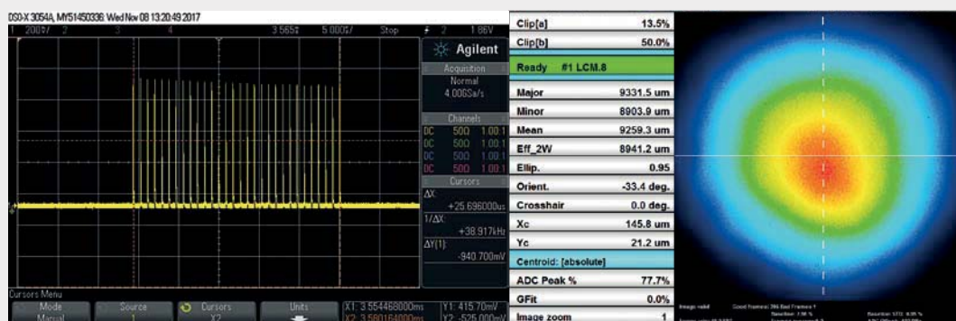
Figure 2 Pump-probe laser output during user experiments in November and December 2017. Left Burst of 30 pulses with a pulse energy of 230 \mu\text{J} at 1.1 MHz. Right Beam profile with >95% Gaussian fit quality.
