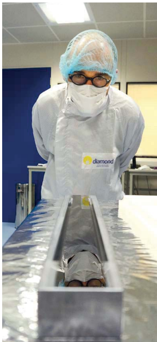
Figure 1 SCS instrument scientist Robert Carley inspects the superpolished X-ray focusing optics from JTEC Corporation at the Diamond Light Source prior to metrology.
