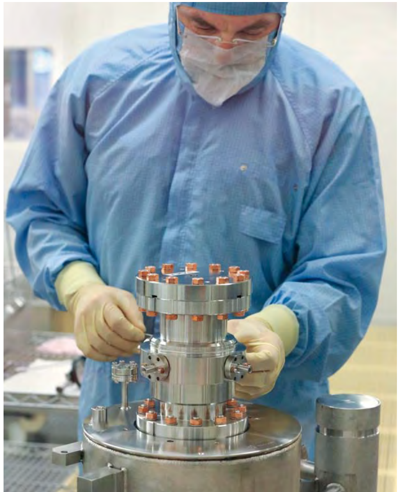
Figure 6 Re-entrant beam position monitor (BPM) assembly to the cold quadrupole (IKC DE17 by DESY)
