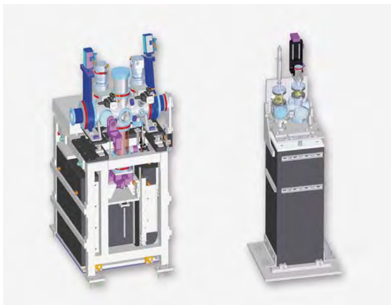
Figure 2 SCS optical laser interfaces. Left SCS laser in-coupling (LIN) Right SCS alignment laser (ALAS)
