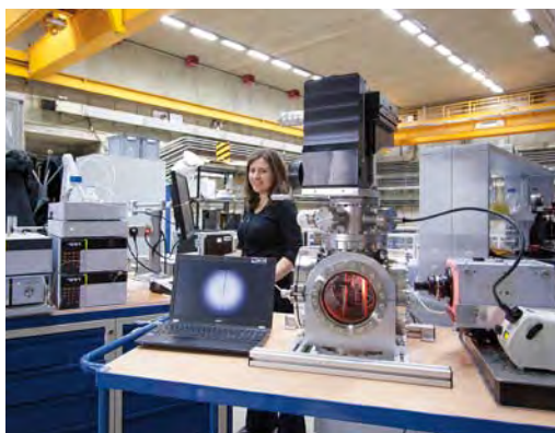
Figure 1 Scientist at the liquid-jet test chamber setup with high-performance liquid chromatography pump system and high-speed camera
