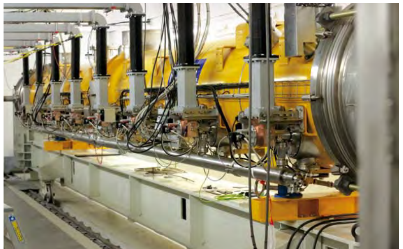
Figure 5 Test of a cryomodule at AMTF (IKC PL05/WP10 by NCBJ)
