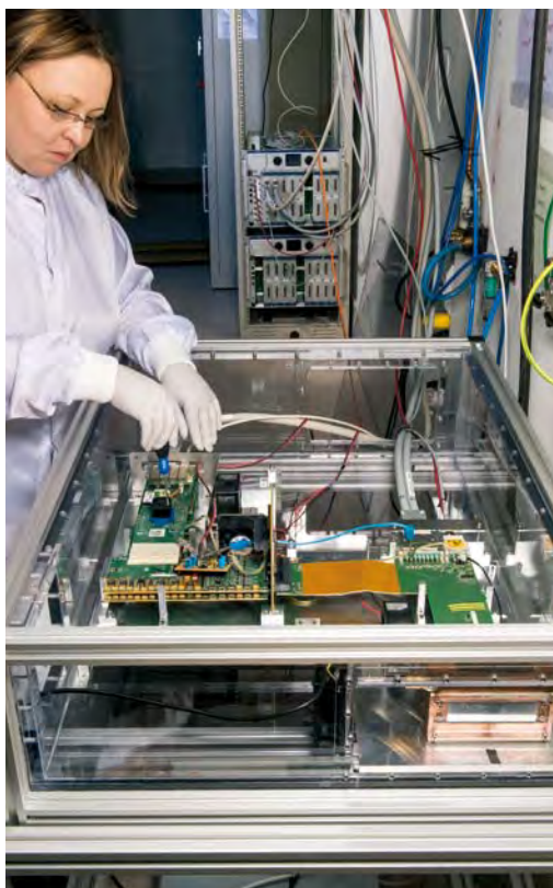
Figure 3 AGIPD single-module prototype installed in an X-ray test stand at European XFEL
