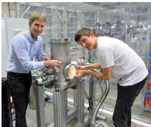
Figure 3 Group members setting up a test vacuum chamber for housing pulsed-coil sample environments
