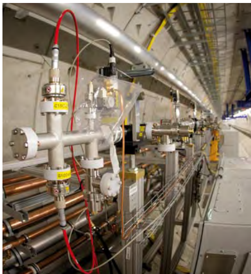
Figure 1 Differential pumping unit upstream of the gas-based diagnostic system, mounted on a custom-made support adapted to the beam height of 2.7 m above the floor at this location in the XTD2 tunnel
