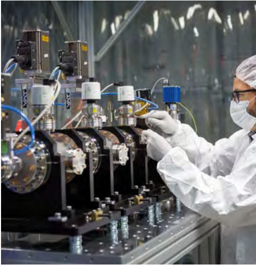
Figure 1 The DPS comprises three sequential vacuum sections
