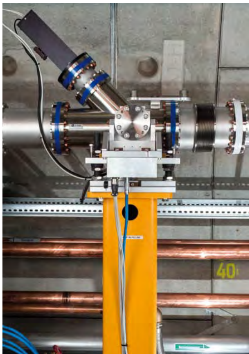
Figure 3 Pop-in monitor Type II-45 in XTD2
