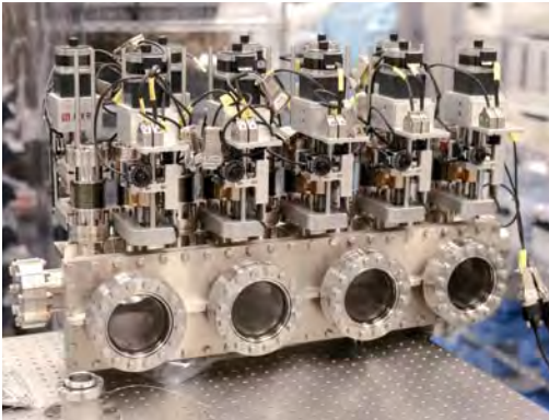
Figure 2 Danish IKC prototype CRL system for the FXE instrument in factory acceptance tests
