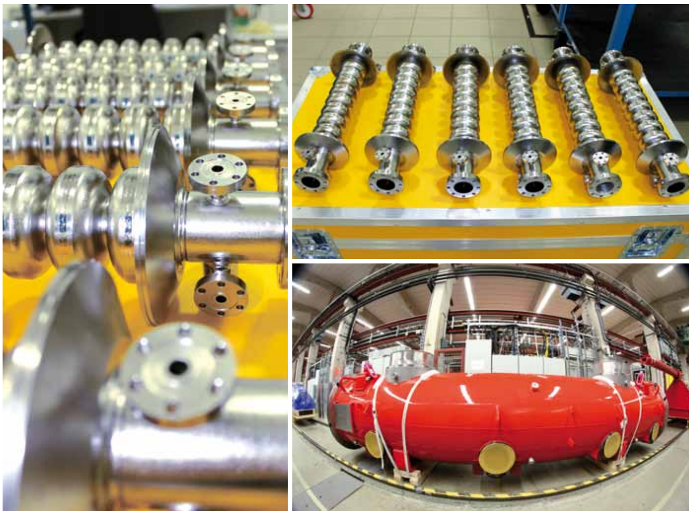
Figure 8 3.9 GHz system. The linearization of the RF-induced curvature in phase space is necessary to preserve the beam quality in the subsequent bunch compressor stages before entering the main linear accelerator. The RF curvature linearization is achieved by a third-harmonic section after the RF gun. The single module at 3.9 GHz consists of eight superconducting RF cavities (IKC IT03/WP46 by INFN – Sezione di Milano, Laboratorio Acceleratori e Superconduttività Applicata (LASA), Italy).
