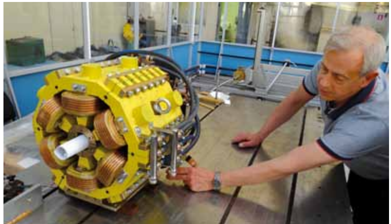
Figure 2 Sextupole magnets. The control of chromatic effects is one of the main issues in the design of the optics in the collimation section. Therefore, introduction of chromaticity-correcting sextupoles becomes essential to improve overall system performance (IKC RU11/WP12 by NIIIEFA).
