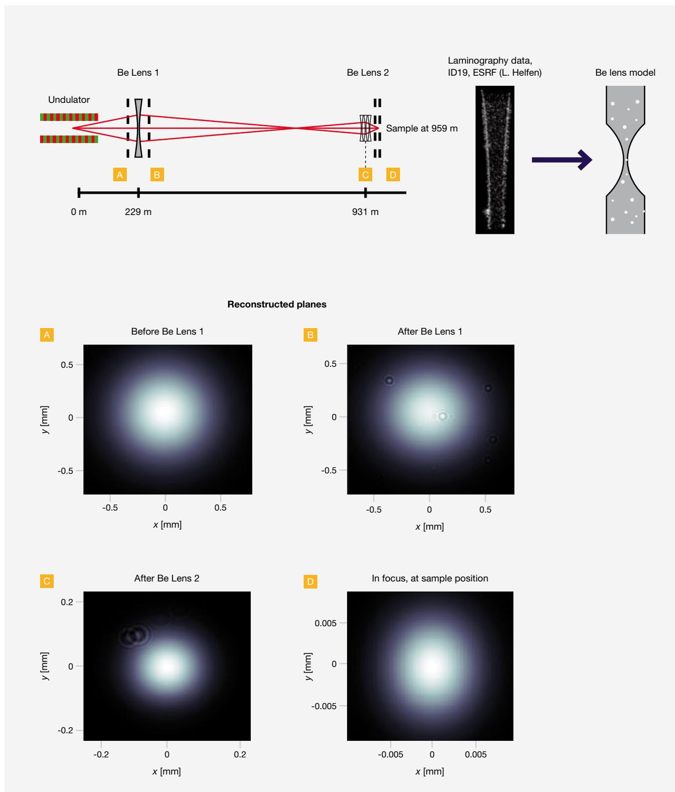
**Figure 1** Schematics of wave field simulations performed in collaboration with Liubov Samoylova from the European XFEL X-Ray Optics and Beam Transport group. The results of computed laminography on beryllium sheets and lenses were important to assess the material quality and build a realistic model for the simulations.
