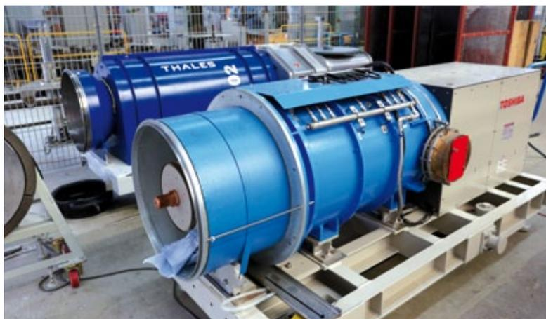
**Figure 2** Klystrons ready for tunnel installation. These special RF sources, which are produced by two different vendors, supply a pulse power of up to 10 MW.
