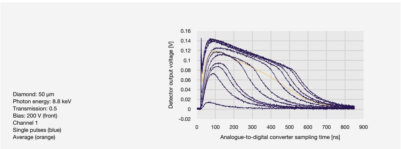
**Figure 3** Diamond detector intensity measurement of single X-ray FEL pulses, showing saturation at higher intensities. Good linearity was observed up to a pulse energy of 1  $\mu\text{J}$ .
