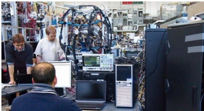
**Figure 2** Operation of the photoelectron spectrometer at DESY's FLASH, synchronized to beam delivery using the European XFEL e-machine timing board and driving a multiboard digitizer readout system
