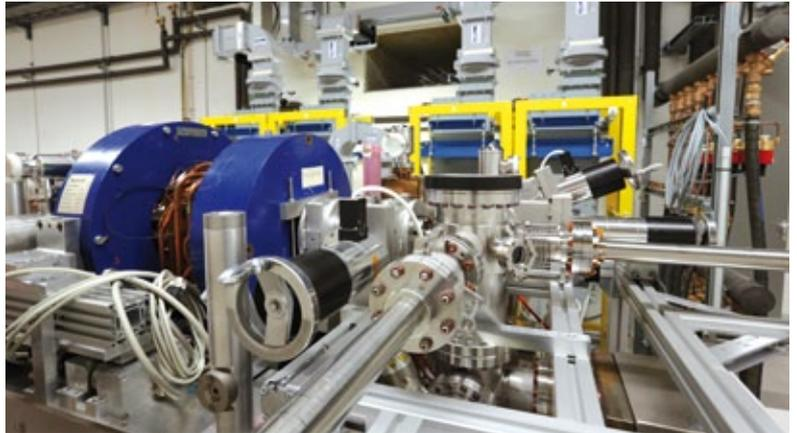
**Figure 6** RF gun installed on the seventh floor of XTIN, with the four waveguides in the background, and the blue solenoid coils surrounding the gun body and the cathode exchange system in the foreground
