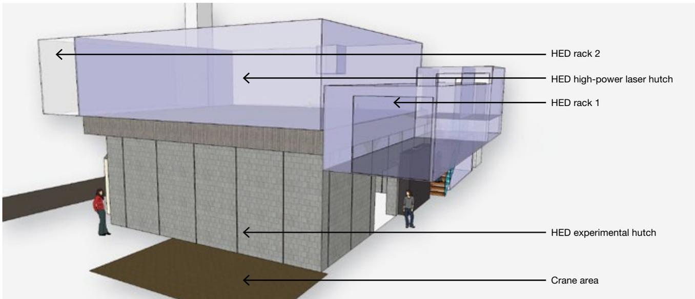
Figure 2 3D model of the enclosure for the HED instrument
