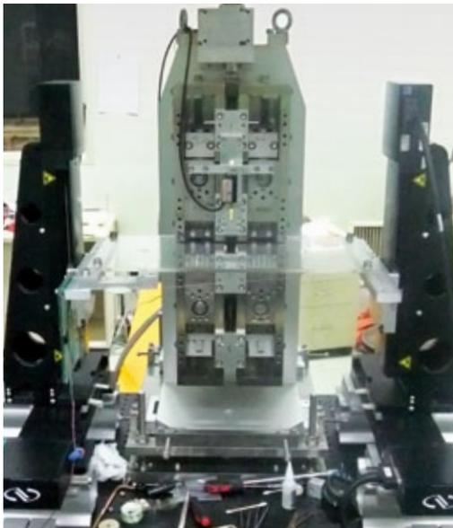
**Figure 2** One of the first phase shifters aligned on a moving wire bench for magnetic tuning
