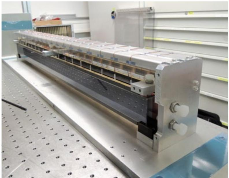
**Figure 1** Prototype of an adaptive mirror. The mirror deflects in horizontal geometry with the deflecting surface facing the camera. Bending can be controlled using piezo elements located at the four edges on the top and bottom of the mirror.
