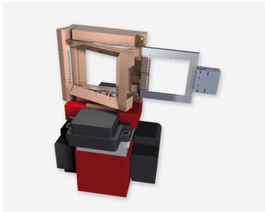
to be conducted at the scientific instruments, he began to develop a common concept for fast sample positioning and a load-lock sample exchange system to be installed at the instruments. The first parts of the prototype sample changer were delivered in December 2013 (Figure 2).
