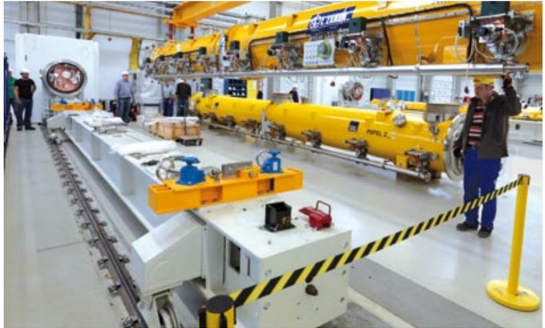
**Figure 1** Accelerator module XM-2 during installation on the AMTF module test stand
