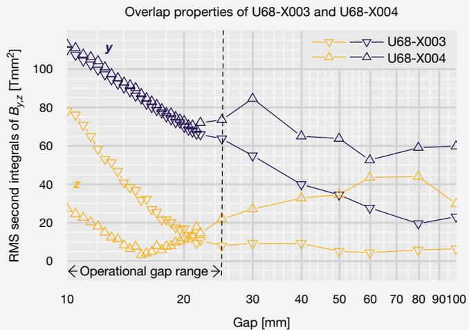
**Figure 1** Magnetic measurement results as a function of gap for two SASE3 U68 undulator segments.
