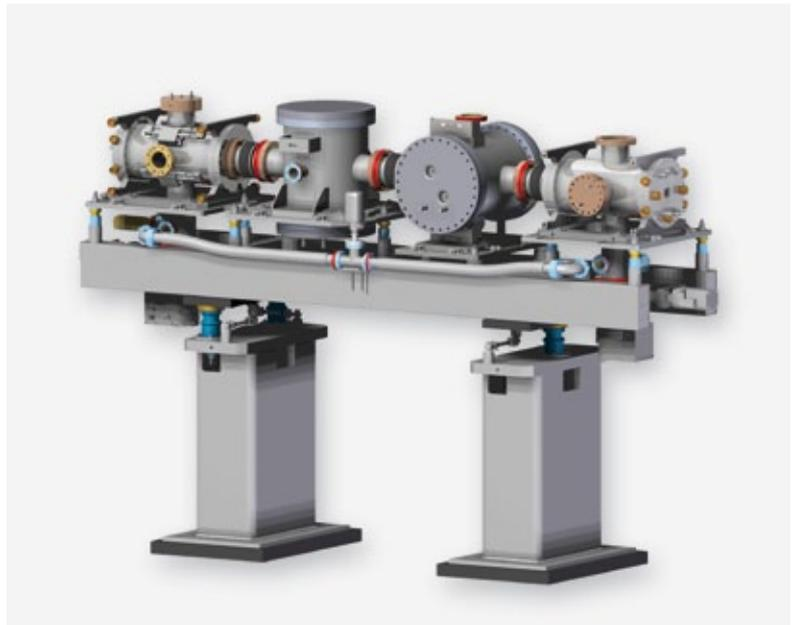
**Figure 1** CAD drawing of the complete X-ray gas monitor, including girder and support pillars
