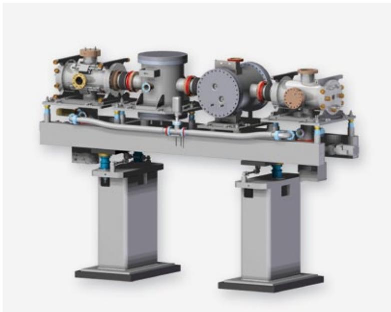
**Figure 1** CAD drawing of the complete X-ray gas monitor, including girder and support pillars
