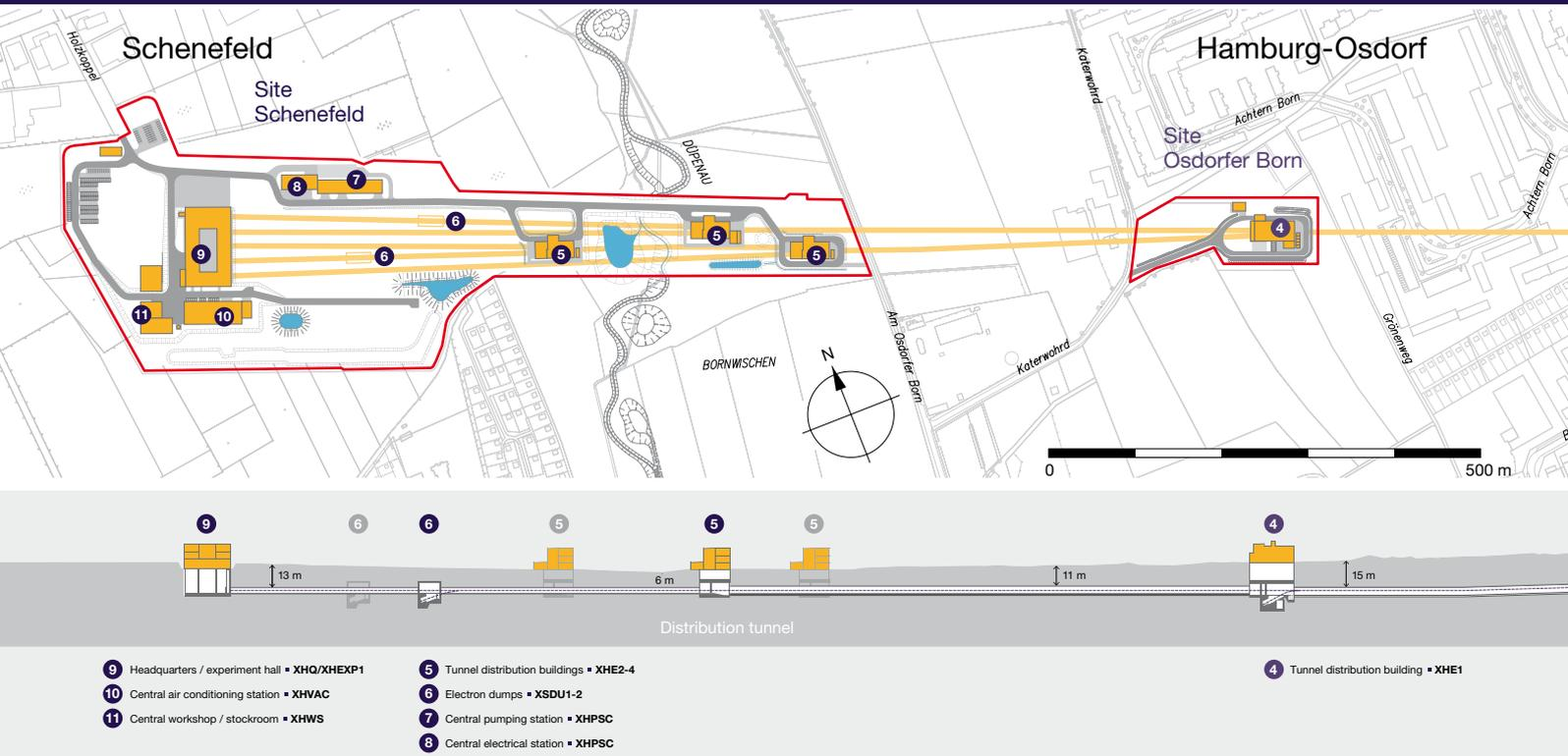
Figure 1 Layout of the European XFEL facility
