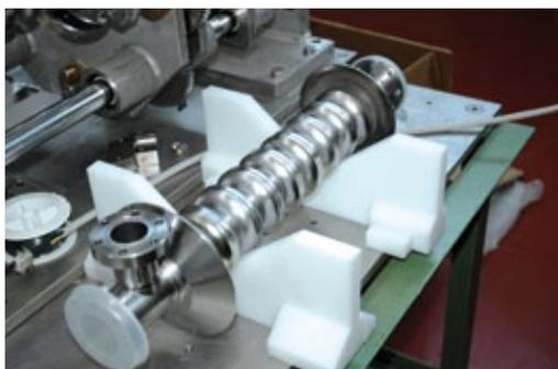
**Figure 7** Producing cavities for the third-harmonic system (IKC IT03 by INFN).
