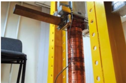
**Figure 3** Tuning the transverse deflecting structure for Bunch Compressor 1 (Contract RU22 to INR)
