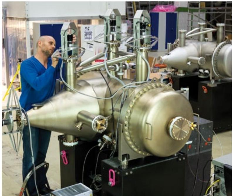
**Figure 2** Mirror chamber for offset and distribution mirrors
