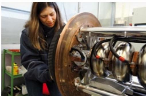
**Figure 5** Manufacturing superconducting niobium cavities (IKC IT01 by INFN)
