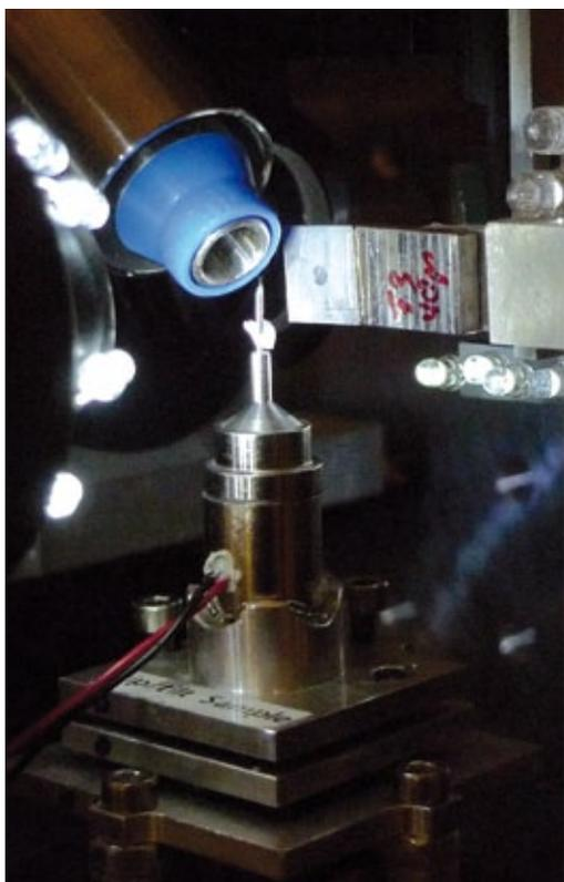
**Figure 2** Sample area setup of a single-particle imaging experiment at Beamline P10 of PETRA III. A single biological cell that has been prepared by rapid freezing in its aqueous environment is kept frozen by a cryostreamer while being imaged using coherent X-rays. The imaging method used here is closely related to those to be used at the SPB instrument.
