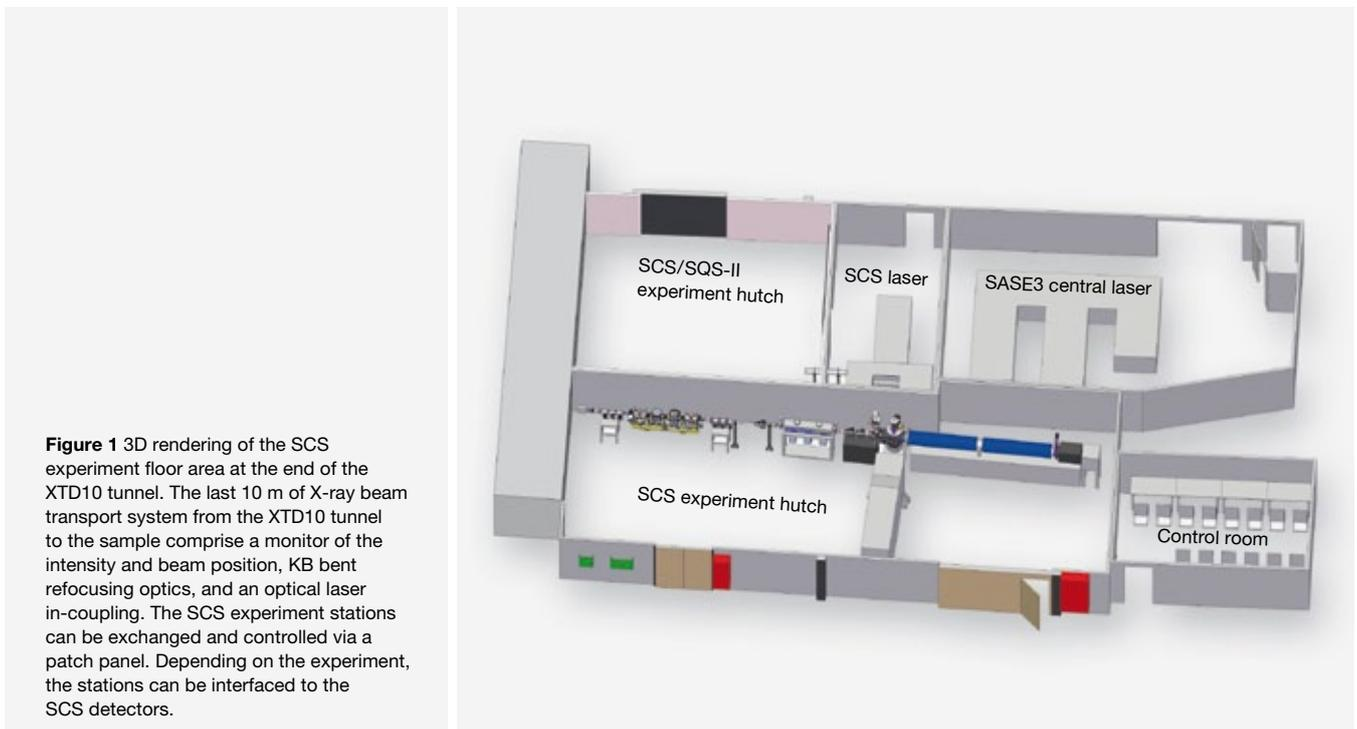
**Figure 1** 3D rendering of the SCS experiment floor area at the end of the XTD10 tunnel. The last 10 m of X-ray beam transport system from the XTD10 tunnel to the sample comprise a monitor of the intensity and beam position, KB bent refocusing optics, and an optical laser in-coupling. The SCS experiment stations can be exchanged and controlled via a patch panel. Depending on the experiment, the stations can be interfaced to the SCS detectors.
