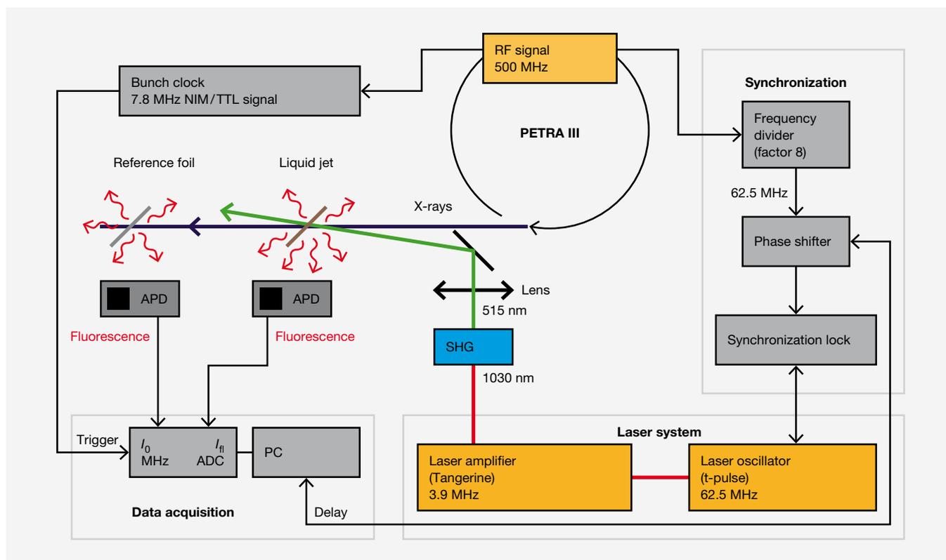
**Figure 3** Schematic layout of the high repetition rate pump-probe experiment using a MHz femtosecond fibre amplifier and a MHz pulse train of hard X-ray pulses from PETRA III.
