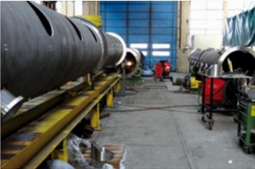
**Figure 6** Manufacturing cryostats for the superconducting modules (IKC IT02 by INFN)
