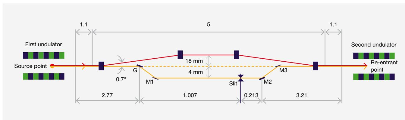
**Figure 1** Schematic layout of the SXRSS setup for the European XFEL, adapted from a working LCLS scheme (G: grating; M: mirror; horizontal distances in metres)
