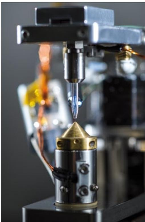
**Figure 1** Liquid-jet system with a 25  $\mu\text{m}$  glass nozzle and the recycling catcher. Both systems are independently exchangeable.
