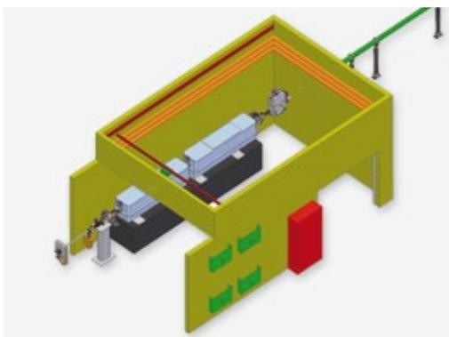
**Figure 1** View of the design of the SPB optics hutch, including two vacuum chambers, each hosting two long X-ray mirrors. These mirrors will be used to produce the 1  $\mu\text{m}$ -scale focus of the SPB instrument.
