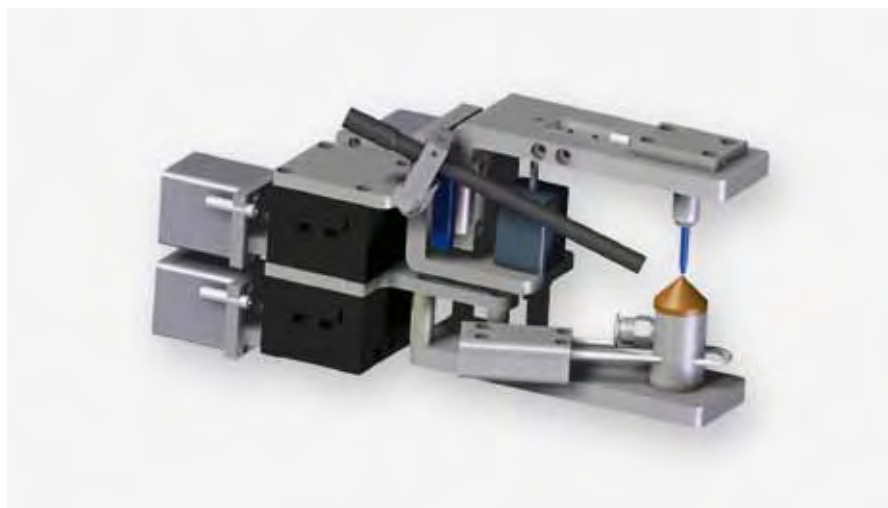
Figure 1 Modular and compact setup for liquid-jet delivery designed by Microliquids GmbH in Göttingen, Germany, in collaboration with the Sample Environment group. Nozzle (blue) and catcher for recovery (copper colour) can be replaced separately. This ensures a versatile setup with state-of-the-art technology for the operation phase of the European XFEL starting in 2016.
