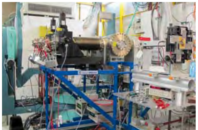
Figure 10 Contract to JINR: Prototype of microchannel plate (MCP)-based detector under test at the DORIS accelerator at DESY
