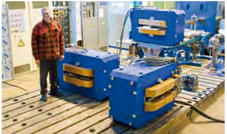
Figure 2 Dipoles for the bunch compressor chicanes at NII-EFA
