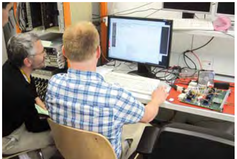
Figure 1 Group members participating in handover tests of the first train builder demonstrator prototype electronics board with one of the development team's firmware specialists. Train builder electronics are developed for the European XFEL at RAL in the UK, and are principally used to acquire and process data from AGIPD, LPD, and DSSC cameras.
