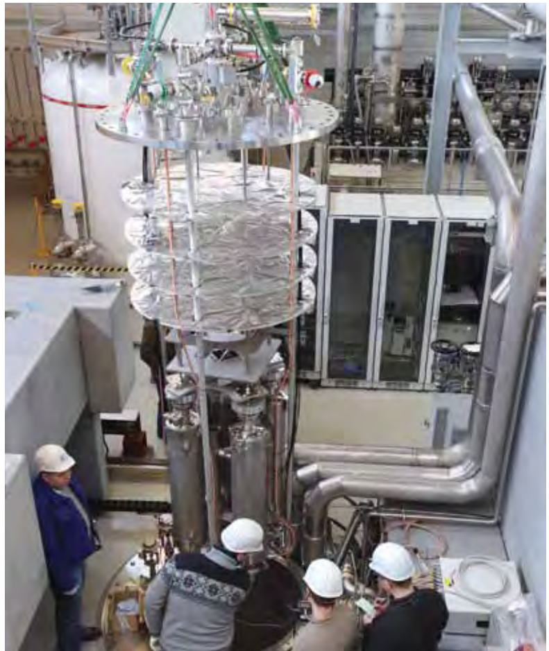
Figure 10 Vertical test cryostats in the AMTF are used to test all 800 superconducting cavities of the European XFEL.
