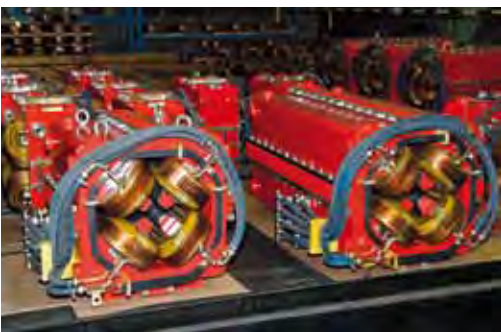
Figure 3 IKC by CIEMAT: Manufacturing the vacuum vessel for the superconducting magnets (left) and integrating a magnet into the vacuum vessel (right) at Trinos Vacuum Projects in Valencia, Spain
