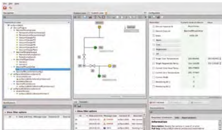
Figure 3 The “default generic GUI” uses all underlying functionalities of Karabo to allow users to configure and control individual and groups of devices.
