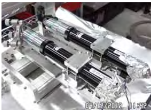
Figure 3 Close-up of two planes of the wavefront measuring device developed in cooperation with the X-Ray Photon Diagnostics group and used at the CXI instrument at LCLS
