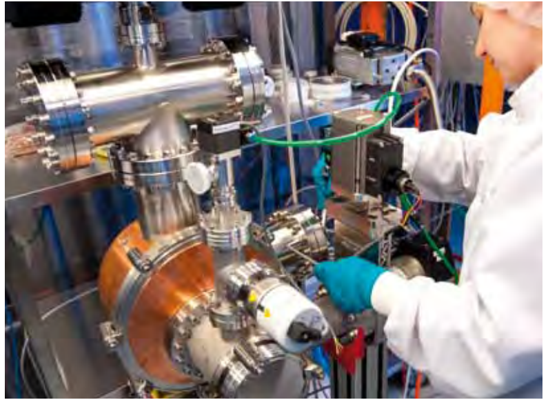
Figure 1 Detector Development group member installing a CCD test setup in the detector laboratory. The detector vacuum vessel (copper cylinder) with cooling (on top of the vacuum vessel) and vacuum system (to the right of the vacuum vessel) is shown.
