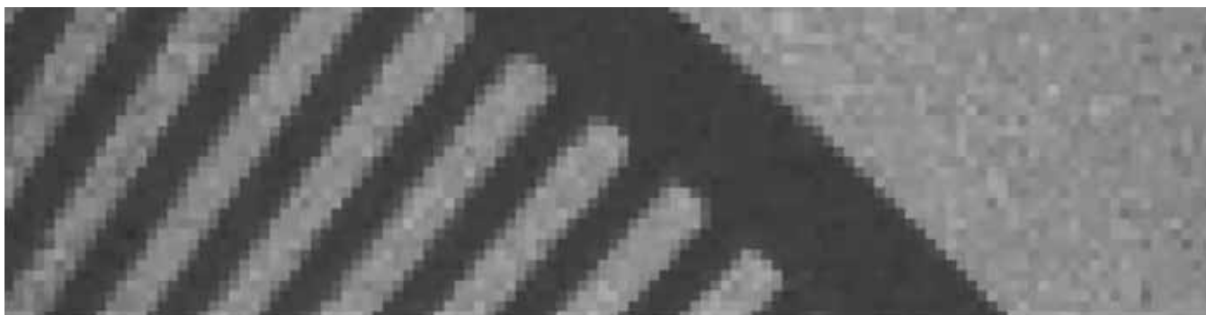
Figure 3 LPD “first light” image taken with a small prototype system. The image is a single frame taken from a movie of a spinning wheel illuminated with X-rays and rotating at a frequency of 45 kHz (light grey: illuminated area; dark grey: shadow cast by the wheel onto the sensor).
