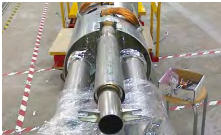
Figure 4 Manufacturing by WUT-WTP of the helium transfer line for AMTF
