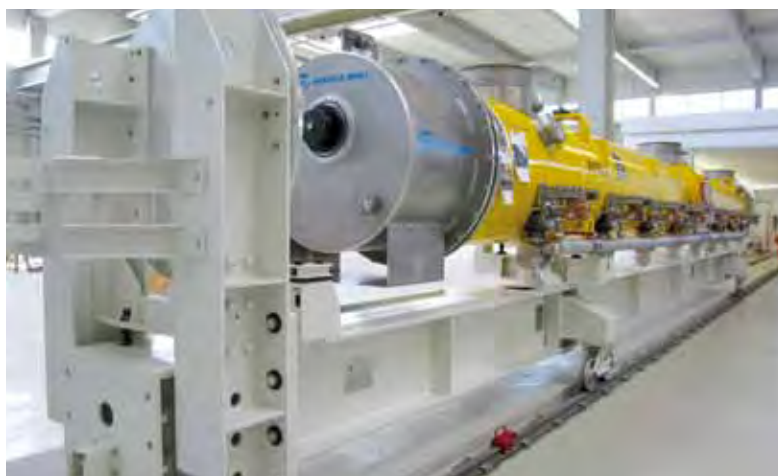
Figure 5 Mobile support by BINP for cryomodule testing in the AMTF hall
