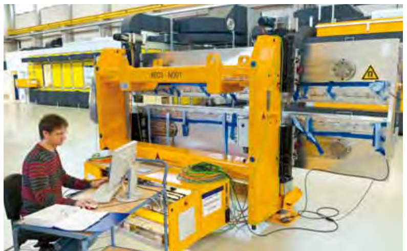
Figure 10 Pre-series prototype of a 5 m undulator segment by CELLS being examined in the European XFEL undulator hall
