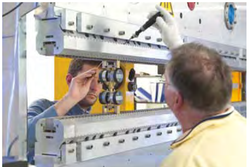
Figure 2 Martin Knoll (left) and Manfred Gaida (right) tune the pole heights of the first U40. For tuning, the gap is fully opened, so the fourfold micrometre dial gauge can be inserted. With this device, the pole height and tilt of the lower pole and the corresponding upper pole can be changed with an accuracy of \pm 1 \mu\text{m} , if needed. One full tuning step requires about one and a half to two days.
