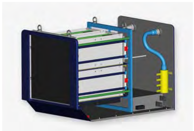
Figure 3 Mechanics concept of a quadrant ( \frac{1}{4} Mpx) LPD system, designed for detector performance and calibration tests
