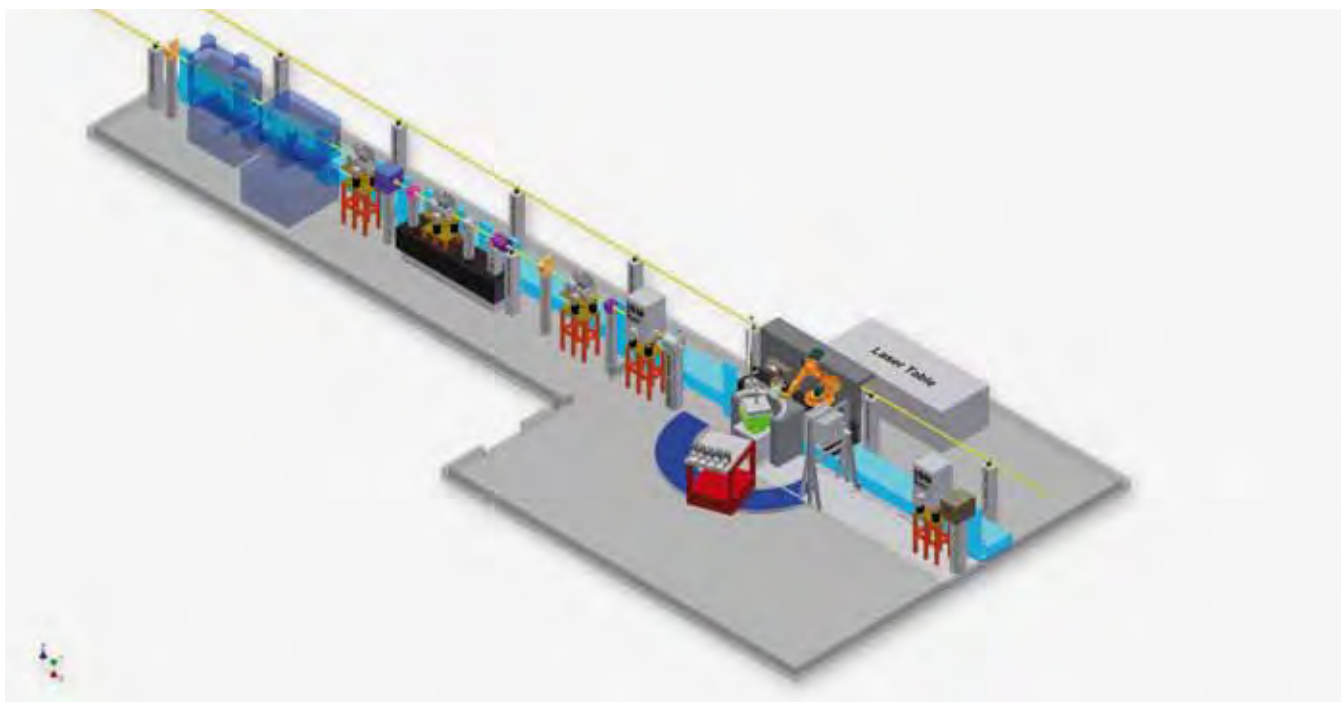
Figure 1 Conceptual design of the FXE instrument in the European XFEL experiment hall behind the SASE1 tunnel (© JJ X-Ray, Denmark)
