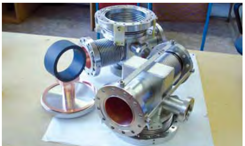
Figure 8 Prototypes of chamber and ceramics of the beamline absorber by NCBJ
