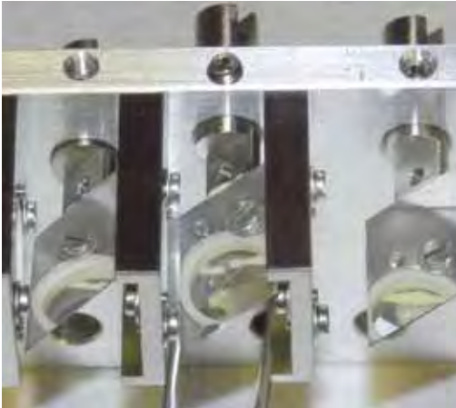
Figure 6 The wavefront imager setup that was engineered by the X-Ray Photon Diagnostics group
