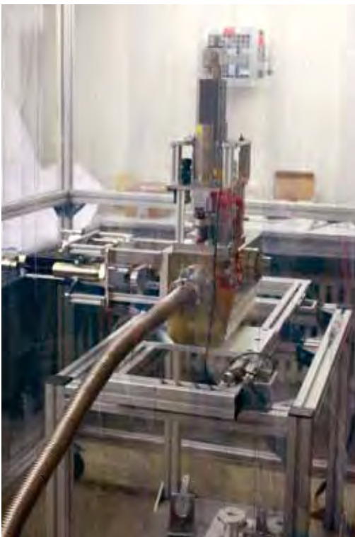
Figure 4 Prototype of the combination of a wire scanner and an optical transition radiation screen
