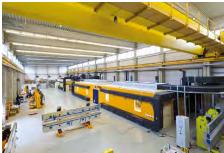
Figure 1 European XFEL magnetic lab in Building 36 with around 1100 m 2 of lab area in December 2011. Five pre-series undulator segments are standing on the left and in the foreground. The three magnetic measurement rooms are in the middle. Room XFEL#1 in the rear is fully operational. Rooms XFEL#2 and XFEL#3 in the foreground (in European XFEL colours) will become operational in spring 2012.
