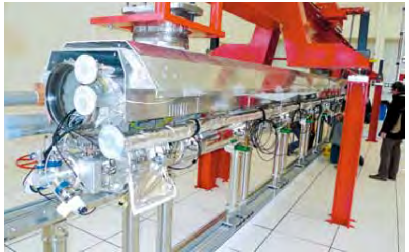
Figure 9 First assembly at CEA (IRFU): cavity string in clean room ISO4 and attached to the supporting structure with helium lines
