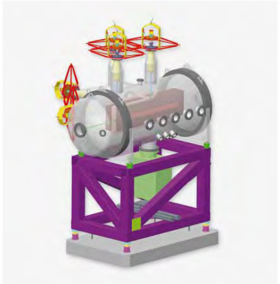
Figure 3 Design of the ultrahigh-vacuum chamber for offset and distribution mirrors (by Tino Noll from HZB and Antje Trapp from European XFEL)
