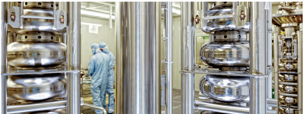
Figure 12: The accelerator technology used in the European XFEL, based on these specialized niobium cavities, has already made an impact on the development of linear accelerators worldwide. Credit: DESY
