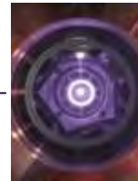
Yb:YAG thin disk multipass
